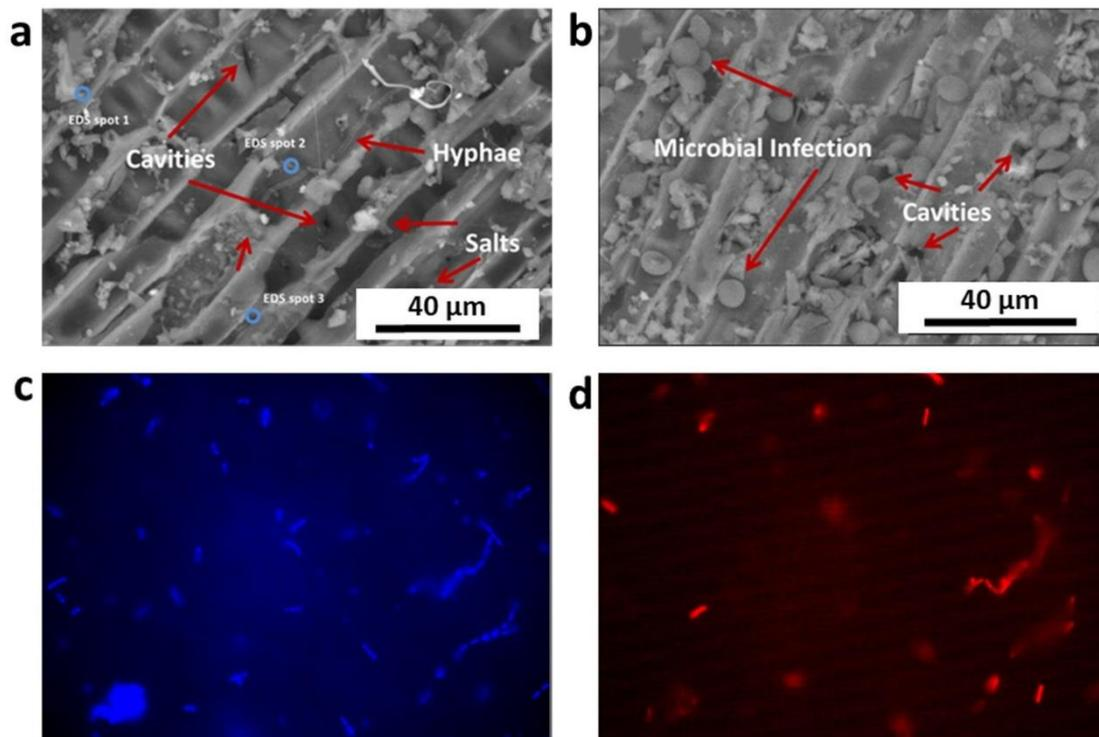
**Figure 5.** (a,b) SEM images (magnification 3000×) of sample #1 (pure core wooden sample, inner the statue). Fungal hyphae (panel (a)) and spores (panel (b)) are visible. (c,d) Images of FISH assays under the epifluorescence microscope using the DAPI-stain for all microbial cells (blue, panel (c)) and the Cy3-labelled EUB probe for *Bacteria* (red, panel (d)) (magnification 1000×).
