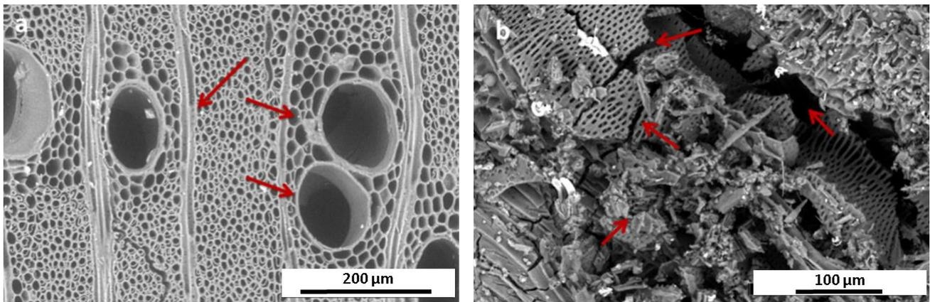
**Figure 6.** (a) SEM image of the *Acacia* standard wood sample (magnification 600×); red arrows indicate the homogeneous structure of wood cell walls. (b) SEM image of the sample #1 (Pure core wooden sample; magnification 800×). The red arrows indicate the strongly fragmented wood structure.
