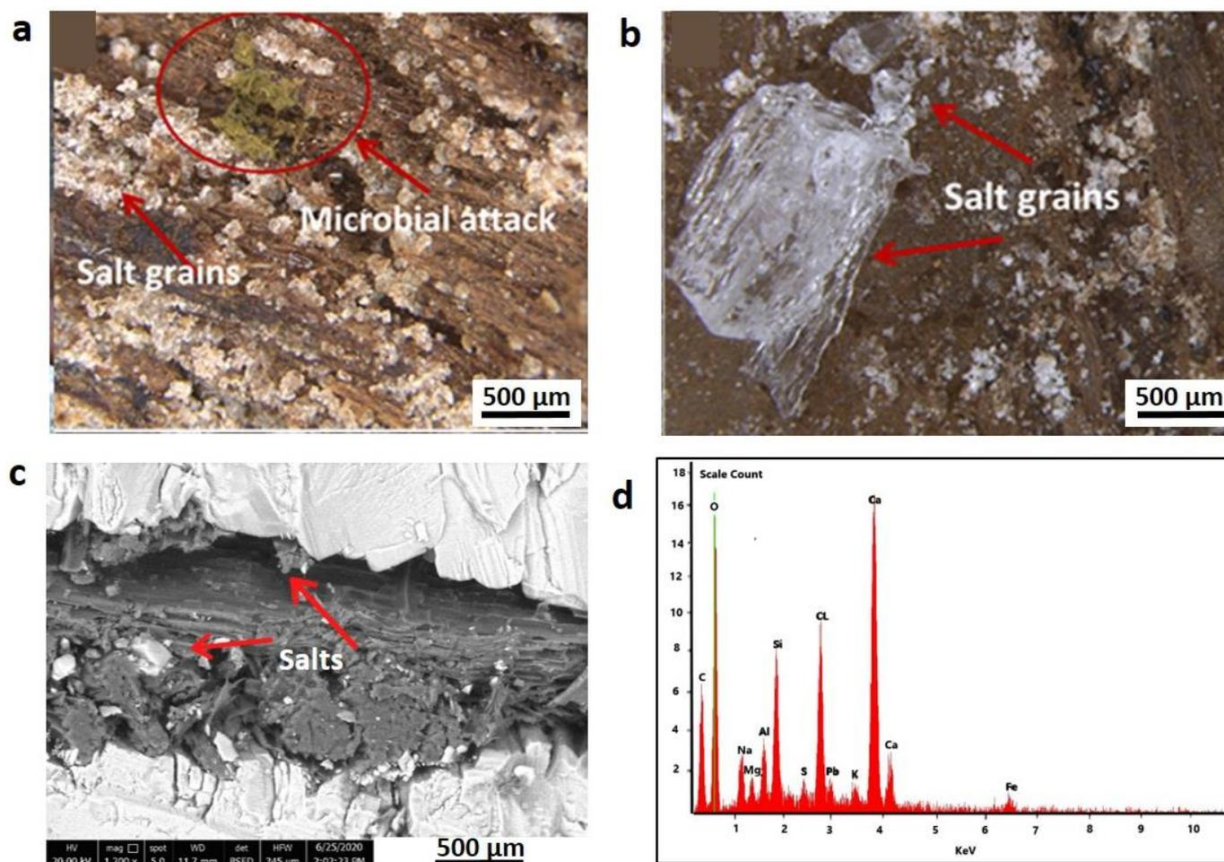
**Figure 3.** (a,b) Stereomicroscopic images (40× magnification) of wood samples #1 (pure core wooden sample) and #2 (wood interfered with soil), of the ancient statue, respectively. Salt grains and a microbial attack are visible. (c) SEM image (magnification 1200×) of sample #2 shows the crystallised salt dispersed on the wood sample. (d) EDX average spectrum of sample #1.
