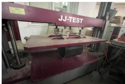
Figure 2. Schematic diagram of PE pipe ring stiffness test.
