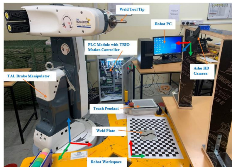
Figure 8. Real-time hardware setup of TAL BRABO manipulator for weld seam detection and tracing.
