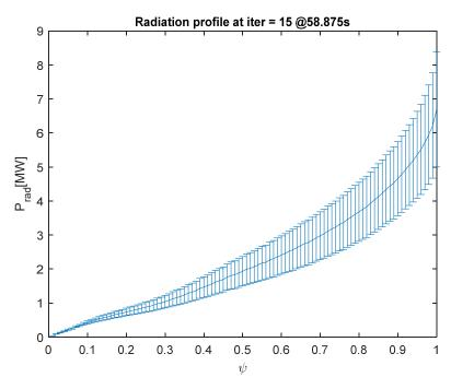
**Figure 7.** Final radiation profile as a function of the flux function  $\psi \in [0,1]$ .
