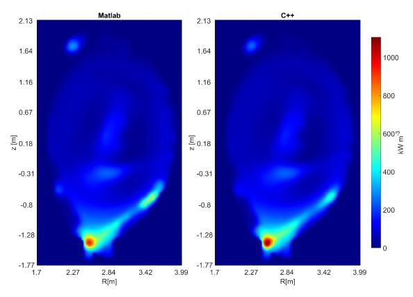
**Figure 9.** Comparison between the final reconstruction (15 iterations) obtained using the original MATLAB code and the C++ implementation, respectively.
