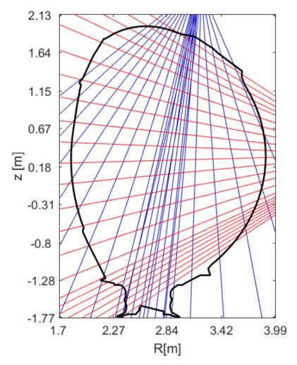
Figure 1. Schematic view of JET bolometric diagnostic layout.
