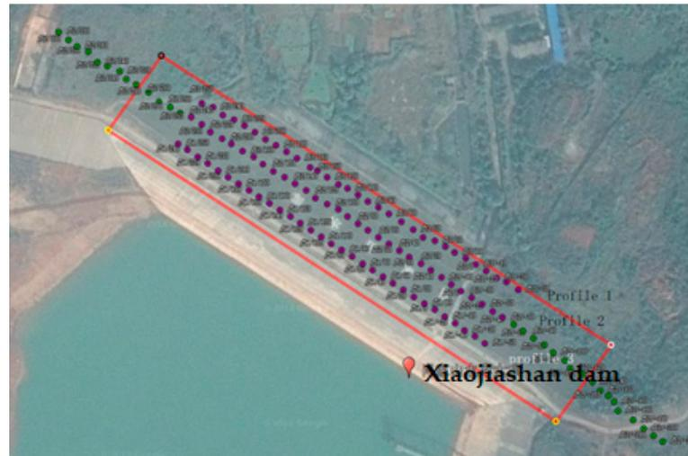
Figure 3. Pseudo-3D arrays for Xiaojiashan Dam leakage detection.
