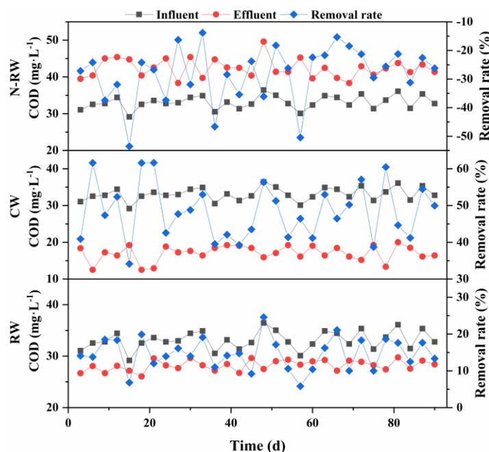
**Figure 5.** Changes of COD concentration and corresponding removal rate in influent and effluent of three groups of wetland systems.
