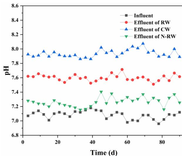
**Figure 6.** Changes of pH in influent and effluent of three groups of wetland systems.
