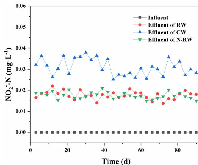
**Figure 4.** Changes of  $\text{NO}_2^- \text{-N}$  concentration in influent and effluent of three groups of wetland systems.
