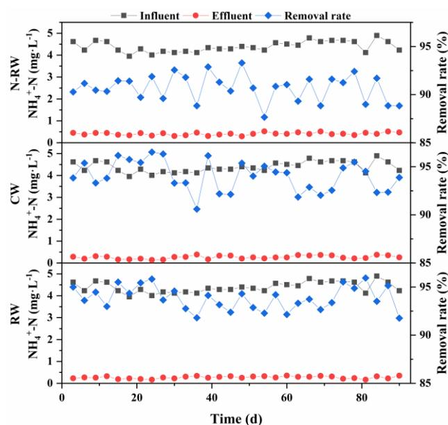
**Figure 2.** Changes of  $\text{NH}_4^+$ -N concentration and corresponding removal rate in influent and effluent of three groups of wetland systems.
