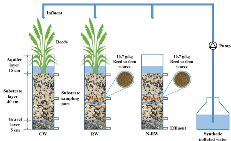
**Figure 1.** Schematic diagram of vertical-flow constructed wetland devices. Note: g/kg—the mass of reed carbon source per kilogram of substrate filler.
