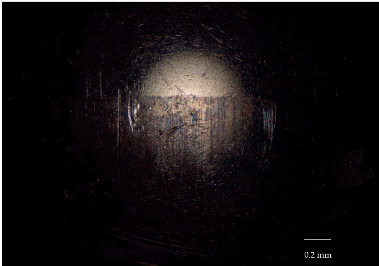
Figure 18. Indenter for test 4, showing no transferred material from the steel sample to the indenter.
