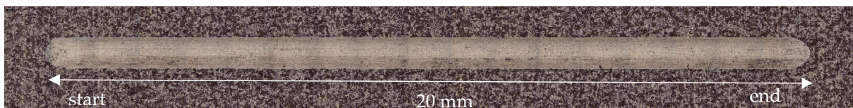
Figure 19. Example scratch from test 4, a steel sample.
