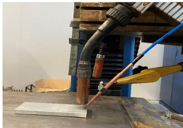
**Figure 5.** Process setup for the admixture of the magnetic powders in the weld pool.
