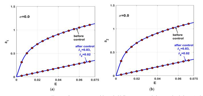
**Figure 22.** *E*—response curve of the studied Jeffcott rotor system before control and after optimal control (i.e.,  $\delta_1 = 0.83$  and  $\delta_2 = 0.02$ ): (a) oscillation amplitude  $a_1$  versus *E* when  $\sigma = 0$ , and (b) oscillation amplitude  $a_2$  versus *E* when  $\sigma = 0$ .
