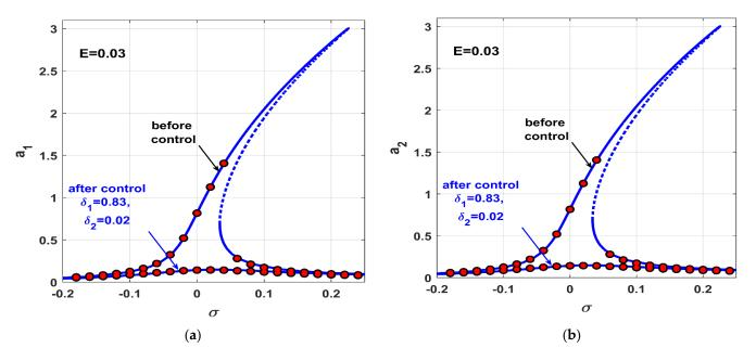
**Figure 20.**  $\sigma$ —response curve of the studied Jeffcott rotor system before control and after optimal control (i.e.,  $\delta_1 = 0.83$  and  $\delta_2 = 0.02$ ): (a) oscillation amplitude  $a_1$  versus  $\sigma$  when E = 0.03, and (b) oscillation amplitude  $a_2$  versus  $\sigma$  when E = 0.03.
