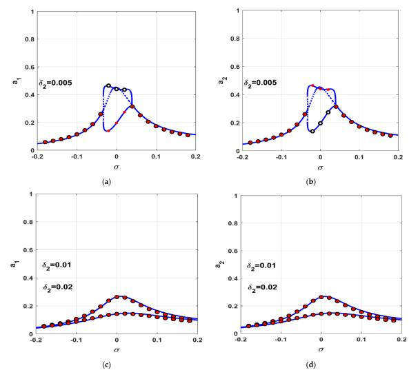
**Figure 15.**  $\sigma$ —response curve of the controlled Jeffcott rotor (i.e., E = 0.03,  $\lambda = 0.05$ , and  $\delta_1 = 0.83$ ) at three different value of the derivative gain  $\delta_2$ : (**a**,**b**) oscillation amplitudes ( $a_1$  and  $a_2$ ) versus  $\sigma$  when  $\delta_2 = 0.005$ , and (**c**,**d**) oscillation amplitudes ( $a_1$  and  $a_2$ ) versus  $\sigma$  when  $\delta_2 = 0.01$ , 0.02.
