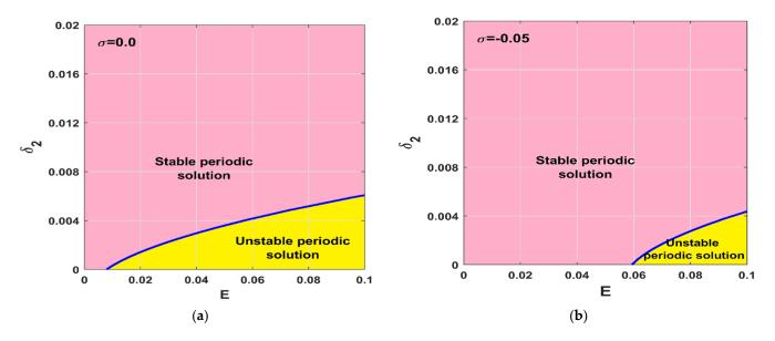
**Figure 19.** Stability charts of the controlled Jeffcott rotor in  $E - \delta_2$  plane when  $\lambda = 0.05$ ,  $\delta_1 = 0.83$ , and  $\delta_2 = 0.002$ : (a) periodic and aperiodic solutions regions in  $E - \delta_2$  plane when  $\sigma = 0$ , (b) periodic and aperiodic solutions regions in  $E - \delta_2$  plane when  $\sigma = -0.05$ .
