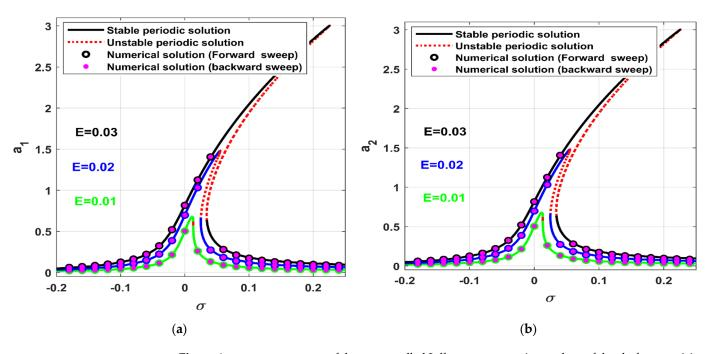
**Figure 4.**  $\sigma$ —response curve of the uncontrolled Jeffcott rotor at various values of the shaft eccentricity *E*: (**a**) oscillation amplitude in *X*—direction (*a*<sub>1</sub>) versus  $\sigma$ , and (**b**) oscillation amplitude in *Y*—direction (*a*<sub>2</sub>) versus  $\sigma$ .
