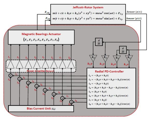
**Figure 3.** Schematic diagram to show the interconnection between the Jeffcott-rotor system, magnetic bearings actuator, and control algorithm.
