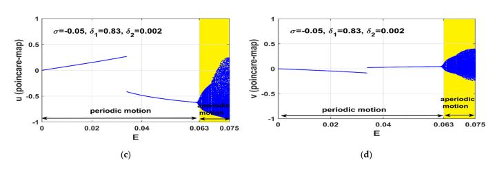
**Figure 11.** *E*—response curve of the controlled Jeffcott rotor (i.e.,  $\delta_1 = 0.83$  and  $\delta_2 = 0.002$ ) and the corresponding bifurcation diagrams at  $\sigma = -0.05$ : (**a**,**b**) oscillation amplitudes ( $a_1$  and  $a_2$ ) versus *E* when  $\sigma = 0$ , and (**c**,**d**) Poincaré-map of the instantaneous oscillations u(t) and v(t) versus *E* when  $\sigma = 0$ .
