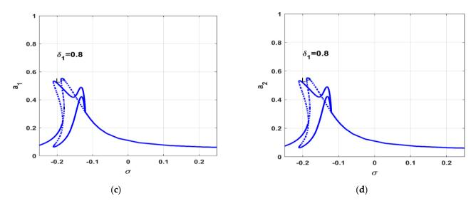
**Figure 13.**  $\sigma$ —response curve of the controlled Jeffcott rotor (i.e., E = 0.03,  $\lambda = 0.05$ , and  $\delta_2 = 0.002$ ) at two different value of the proportional gain  $\delta_1$ : (**a**,**b**) oscillation amplitudes ( $a_1$  and  $a_2$ ) versus  $\sigma$  when  $\delta_1 = 0.85$ , and (**c**,**d**) oscillation amplitudes ( $a_1$  and  $a_2$ ) versus  $\sigma$  when  $\delta_1 = 0.8$ .
