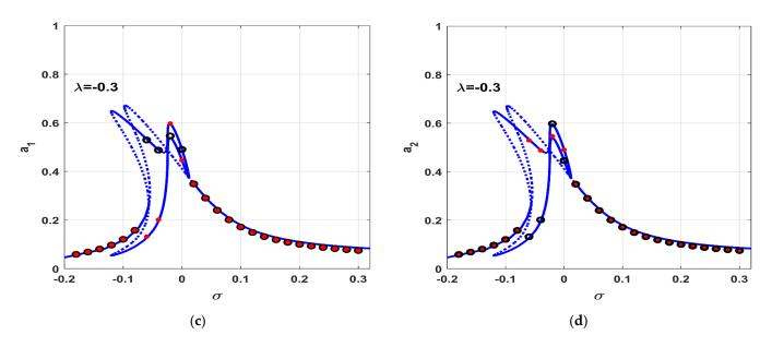
**Figure 12.**  $\sigma$ —response curve of the controlled Jeffcott rotor (i.e., E = 0.03,  $\delta_1 = 0.83$ , and  $\delta_2 = 0.002$ ) at the negative and positive non-linear stiffness coefficient ( $\lambda$ ): (**a**,**b**) oscillation amplitudes ( $a_1$  and  $a_2$ ) versus  $\sigma$  when  $\lambda = 0.3$ , and (**c**,**d**) oscillation amplitudes ( $a_1$  and  $a_2$ ) versus  $\sigma$  when  $\lambda = -0.3$ .
