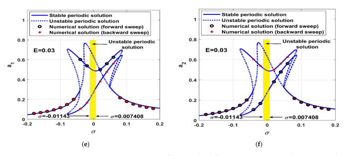
**Figure 6.**  $\sigma$ —response curve of the controlled Jeffcott rotor (i.e.,  $\delta_1 = 0.83$ , and  $\delta_2 = 0.002$ ) at three different values of the shaft eccentricity *E*: (**a**,**b**) oscillation amplitudes ( $a_1$  and  $a_2$ ) versus  $\sigma$  when E = 0.01, (**c**,**d**) oscillation amplitudes ( $a_1$  and  $a_2$ ) versus  $\sigma$  when E = 0.02, and (**e**,**f**) oscillation amplitudes ( $a_1$  and  $a_2$ ) versus  $\sigma$  when E = 0.03.
