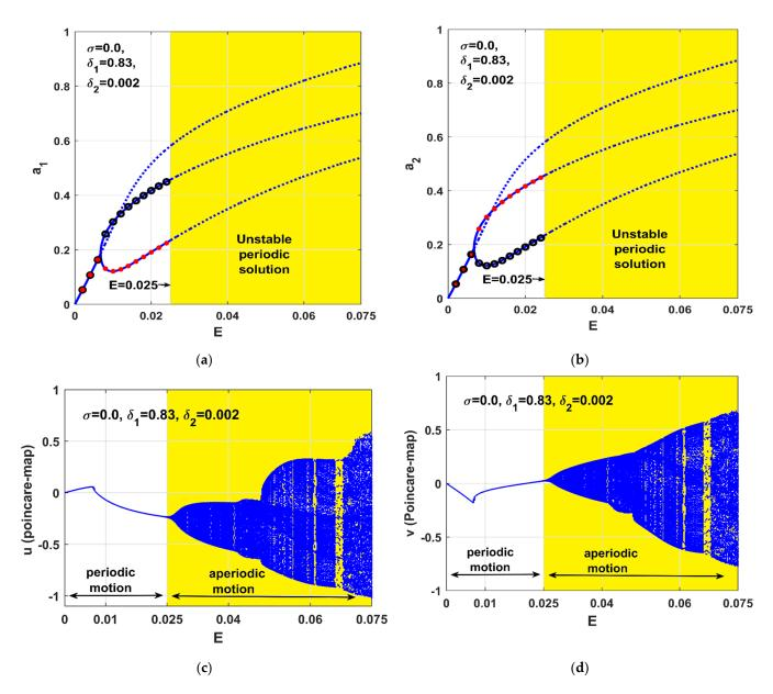
**Figure 7.** *E*—response curve of the controlled Jeffcott rotor (i.e.,  $\delta_1 = 0.83$  and  $\delta_2 = 0.002$ ) and the corresponding bifurcation diagrams at  $\sigma = 0.0$ : (**a**,**b**) oscillation amplitudes ( $a_1$  and  $a_2$ ) versus *E* when  $\sigma = 0$ , and (**c**,**d**) Poincaré-map of the instantaneous oscillations u(t) and v(t) versus *E* when  $\sigma = 0$ .
