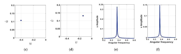
**Figure 8.** Periodic time-response, Poincaré-map, and frequency-spectrum of the controlled Jeffcottrotor according to Figure 7 (i.e., at  $\sigma = 0$ ,  $\delta_1 = 0.83$ ,  $\delta_2 = 0.002$ ) when E = 0.02: (**a**,**b**) the normalized temporal oscillations u(t) and v(t) in X and Y direction, (**c**,**d**) the corresponding Poincaré-map, (**e**,**f**) the corresponding frequency-spectrum.
