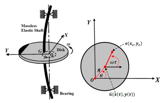
Figure 1. Uncontrolled Jeffcott rotor system.
