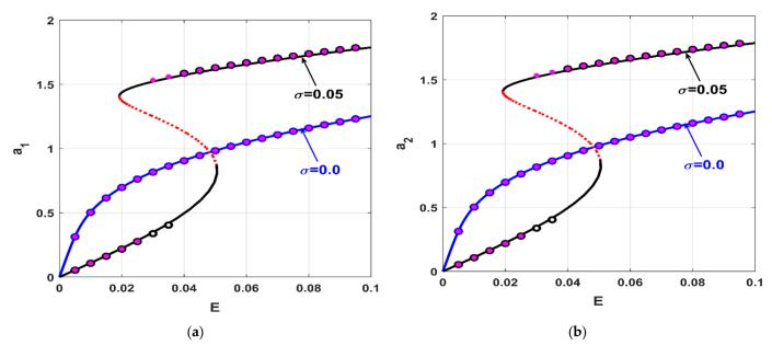
**Figure 5.** *E*—response curves of the uncontrolled Jeffcott rotor at various values of  $\sigma$ : (**a**) oscillation amplitude in *X*—direction (*a*<sub>1</sub>) versus the eccentricity (*E*), and (**b**) oscillation amplitude in *Y*—direction (*a*<sub>2</sub>) the eccentricity (*E*).
