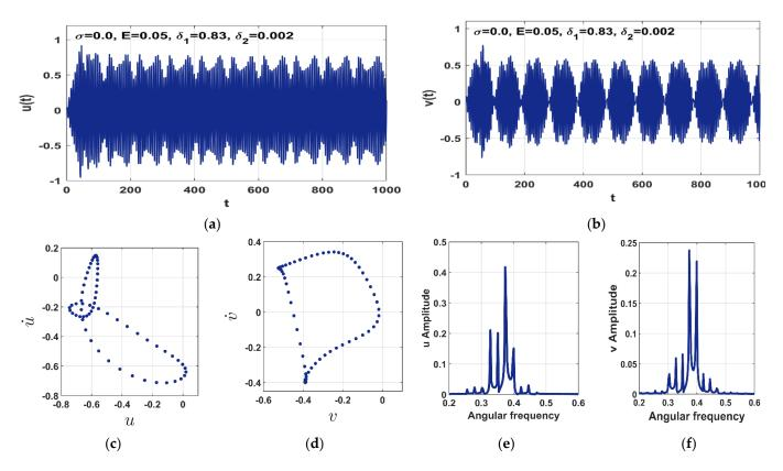
**Figure 9.** Quasi-periodic time-response, Poincaré-map, and frequency-spectrum of the controlled Jeffcott-rotor according to Figure 7 (i.e., at  $\sigma = 0$ ,  $\delta_1 = 0.83$ ,  $\delta_2 = 0.002$ ) when E = 0.05: (**a**,**b**) the normalized temporal oscillations u(t) and v(t) in *X* and *Y* direction, (**c**,**d**) the corresponding Poincaré-map, (**e**,**f**) the corresponding frequency-spectrum.
