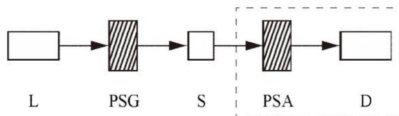
**Figure 1.** Stokes vector measurement system (in dotted box). L: light source, PSG: polarizer, S: sample; PSA: polarizer, D: light intensity detector.
