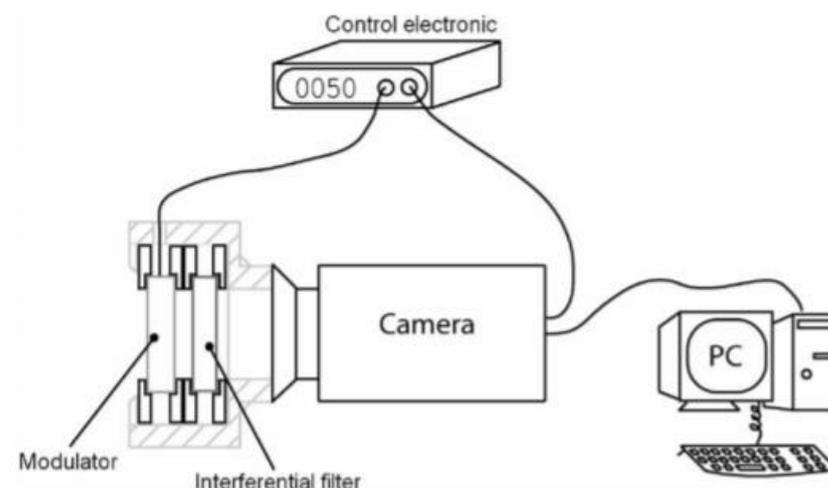
**Figure 4.** Schematic diagram of fixed variable delay wave plate [20].
