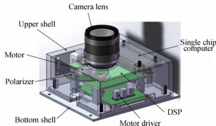
**Figure 2.** Structural design of rotary polarization imaging polarization camera [15].
