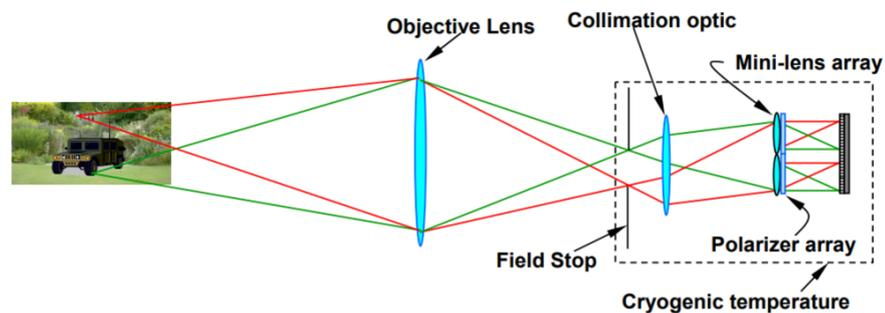
Figure 8. Schematic diagram of polarization imaging with sub-aperture [29].
