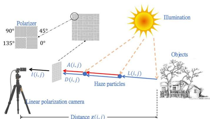
**Figure 10.** The physical model of atmospheric scattering and polarimetric imaging.  $L(i, j)$ : non-polarized light,  $A(i, j)$ : Airlight,  $D(i, j)$ : direct light,  $I(i, j)$ : the irradiance [51].
