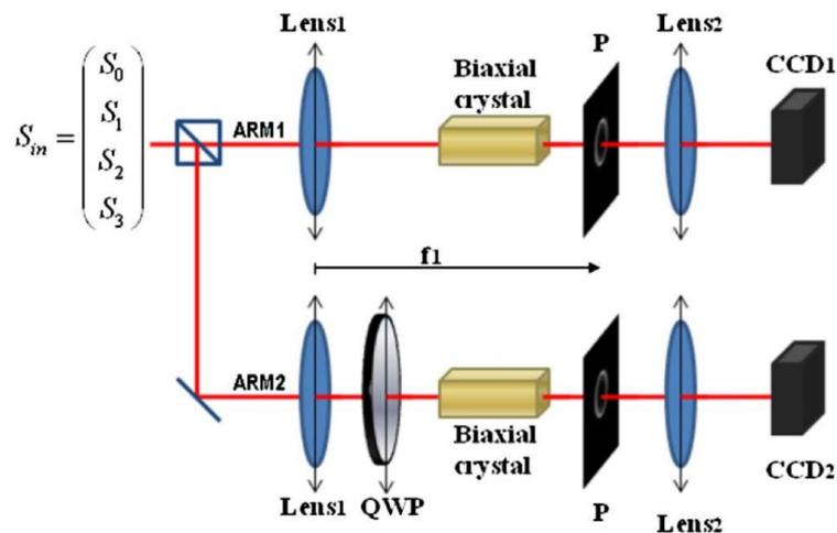
Figure 7. Schematic diagram of fractional amplitude polarization imaging [28].
