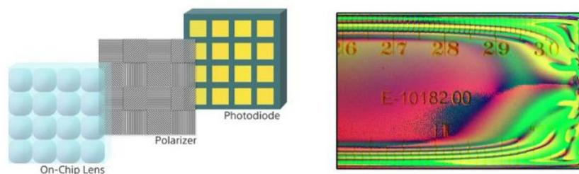
**Figure 9.** Structure of the split-focal plane polarization sensor IMX250 MZR. Right: Internal stress of a transparent ruler made visible by false color presentation of the polarization [42].
