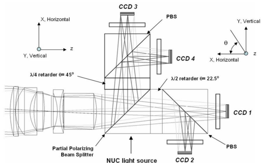
Figure 6. Schematic diagram of full polarization state of fractional amplitude measurement [27].
