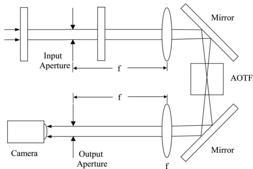
**Figure 5.** System principle diagram of imaging spectral polarizer based on acousto-optic filter type and liquid crystal phase tunable [21].
