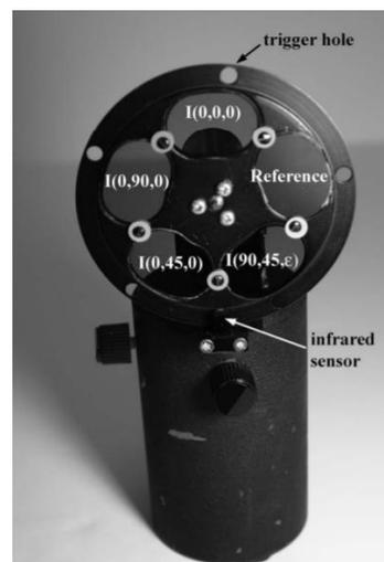
**Figure 3.** High-speed non-simultaneous polarization imaging system [16].
