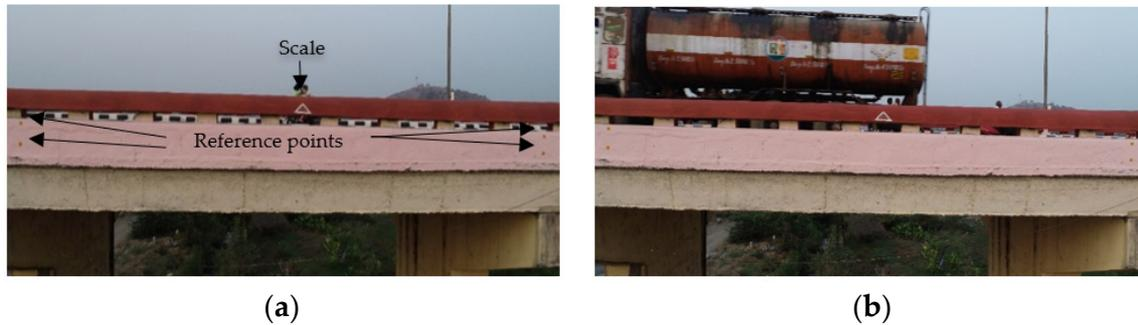
**Figure 11.** UAV images acquisition (a) prior to vehicle passage and (b) during vehicle passage.
