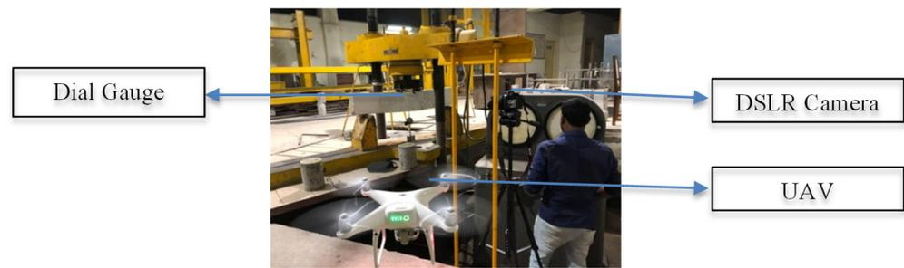
**Figure 4.** Image acquisition using DSLR camera and UAV during loading.
