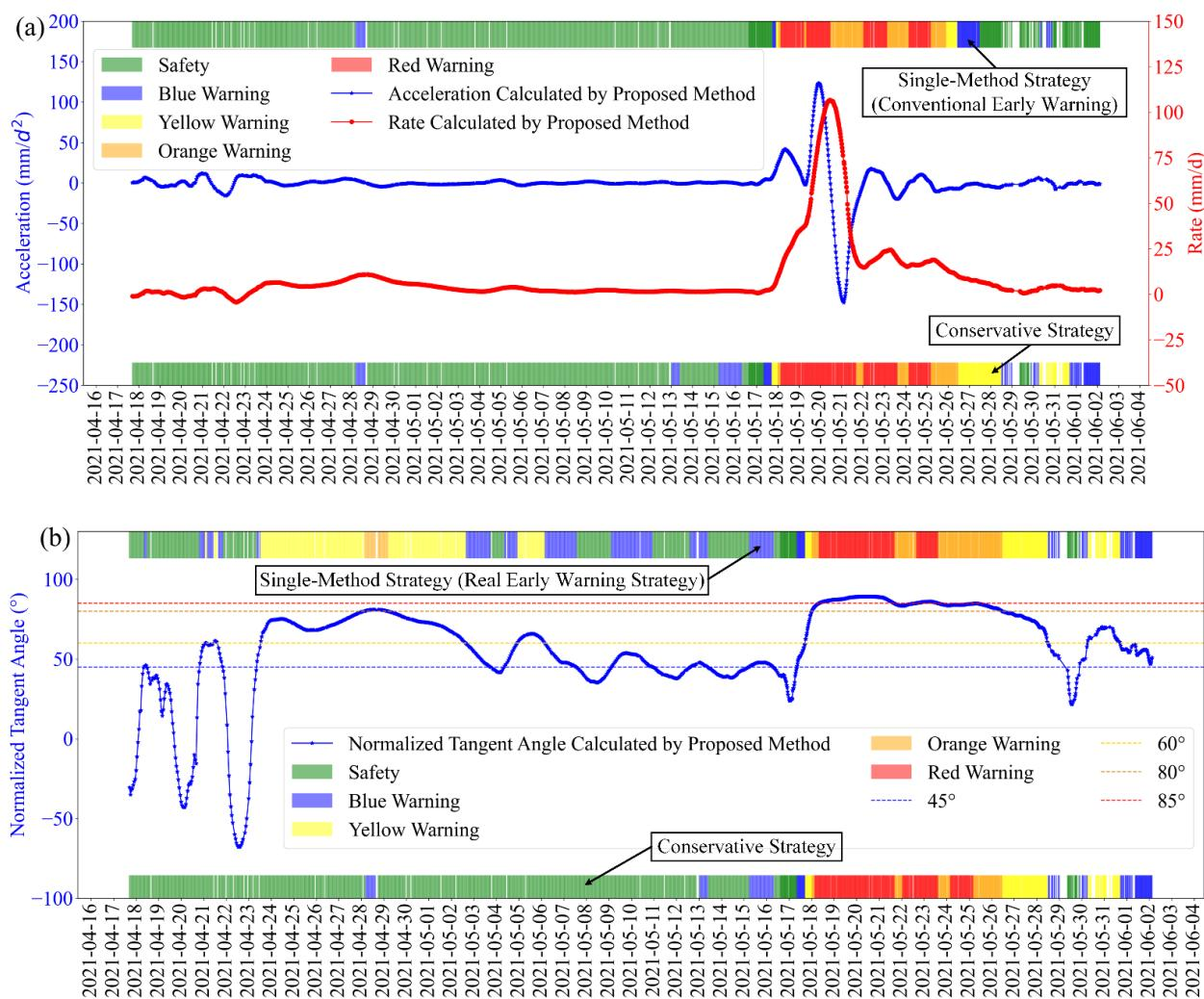
**Figure 7.** Early warning results of the LISHAN-DB02 monitoring station obtained by the proposed method. (a) Results of the conventional warning method based on velocity and acceleration. (b) Results of the critical sliding warning method based on the normalized tangent angle.
