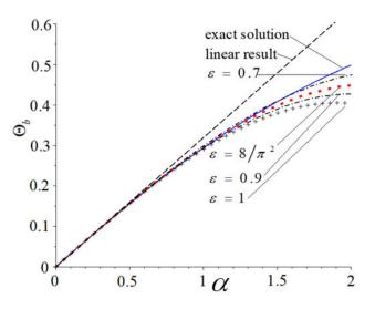
**Figure 2.** Rotation angle at free end vs. point force for different  $\varepsilon$ .
