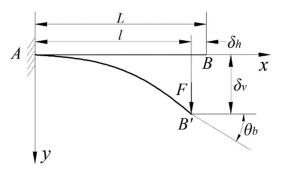
Figure 1. Large deformation of beam under point load at free end.
