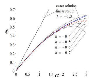
Figure 3. Rotation angle at free end vs. point force when h takes different values.
