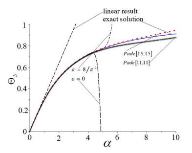
Figure 4. Thirieth solution to rotation angle at the free end vs. point force.
