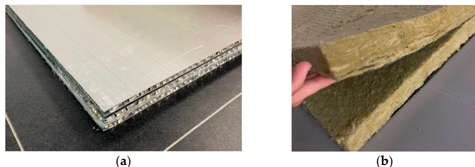
Figure 1. Traditional solution components: (a) honeycomb aluminum panels; (b) mineral wool layer.
