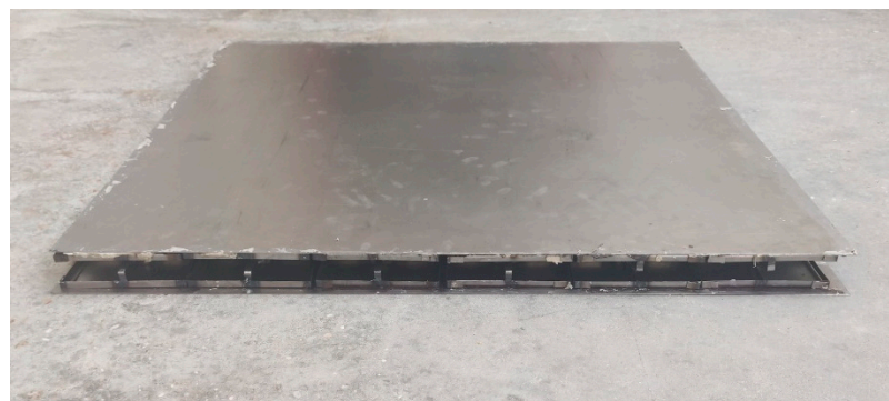
Figure 8. Tested Metasolution sample consisting of the combination of elastic structure and external steel panels.
