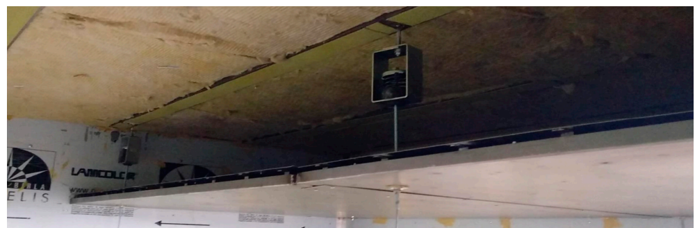
Figure 12. Deck covering mock-up with the 450 mm air-gap configuration.
