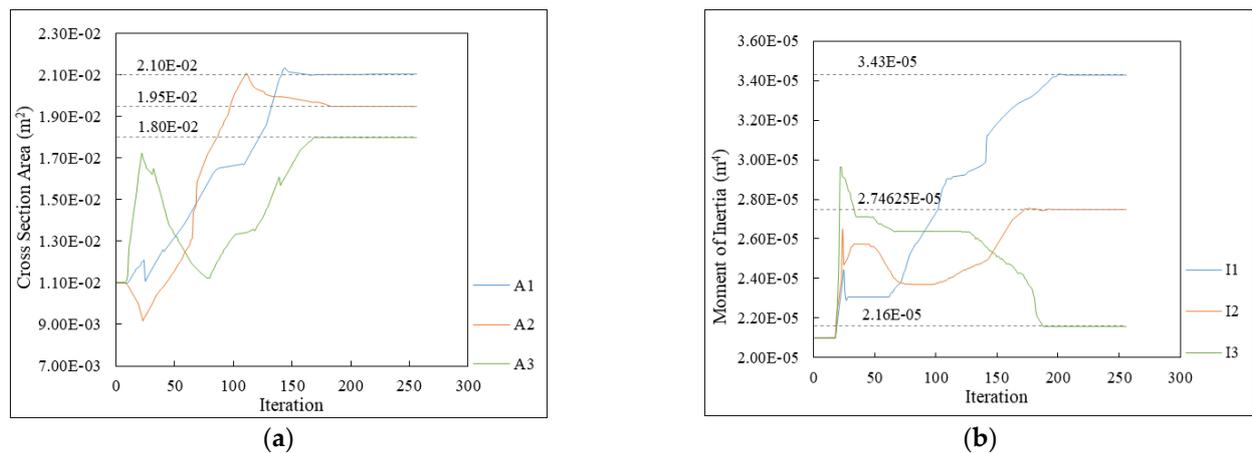
**Figure 5.** Cross-sectional area and moment of inertia as a function of the number of iterations. (a) Cross-sectional area; (b) Moment of inertia.
