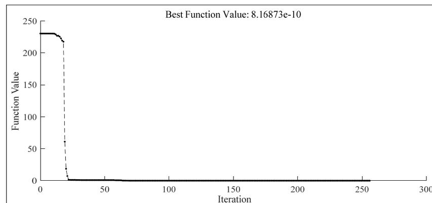
**Figure 6.** Function value for rigid frame damage identification.
