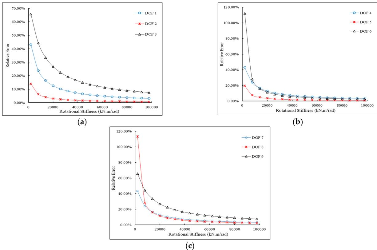
Figure 9. Nodal displacement error caused by different nodal rotational stiffnesses. (a) Degree of Freedom 1–3; (b) Degree of Freedom 4–6; (c) Degree of Freedom 7–9.
