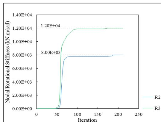
Figure 10. Nodal rotational stiffness as a function of the number of iterations.
