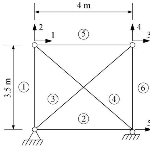
Figure 1. Six-member truss.
