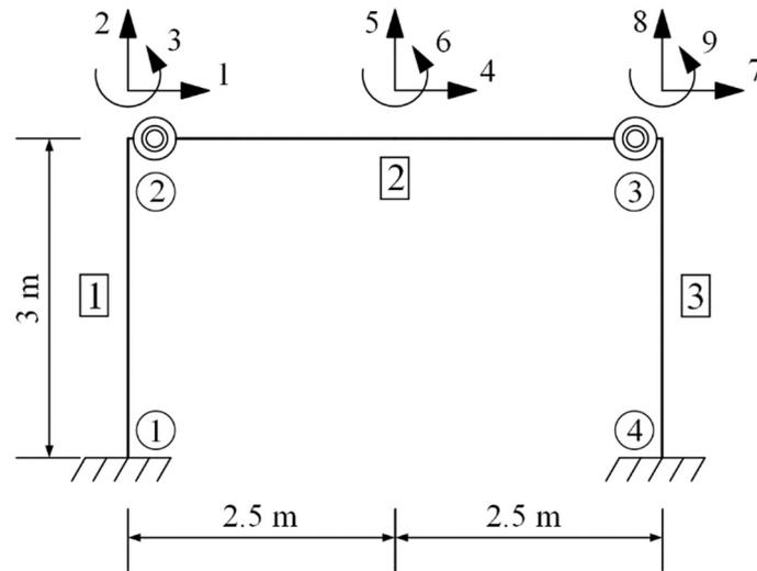
Figure 8. Three-member semi-rigid frame example.
