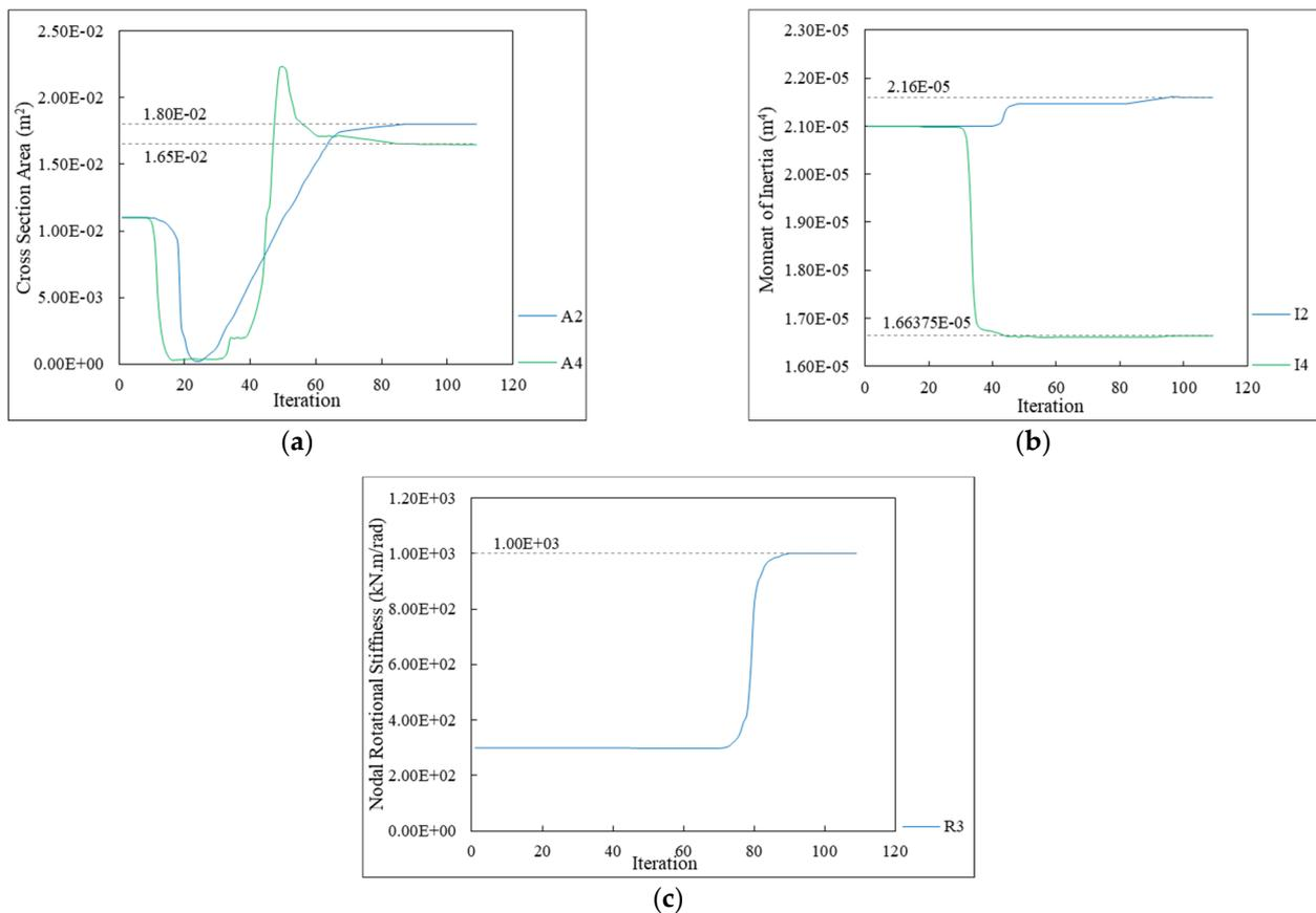
**Figure 13.** Cross-sectional area, moment of inertia, and nodal rotational stiffness as a function of the number of iterations. (a) Cross-sectional area; (b) Moment of inertia; (c) Nodal rotational stiffness.
