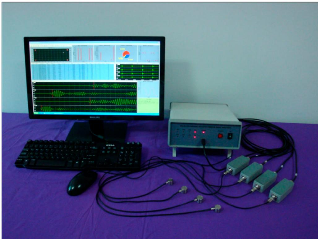
**Figure 1.** 8- channel DS2-B series acoustic emission testing system.
