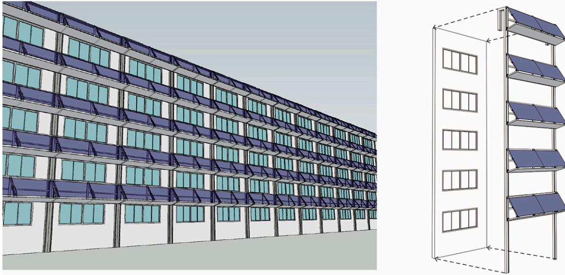
**Figure 9.** Simulation image of kinetic façade system installed on Won-Hyo Elementary School.
