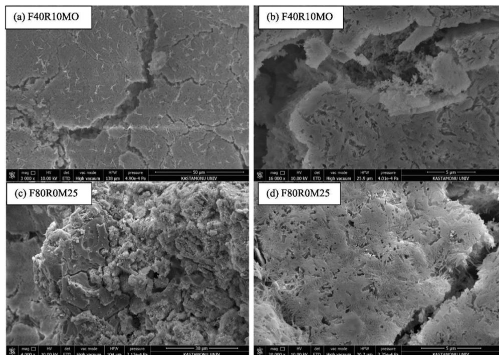
**Figure 11.** SEM images of foam concrete samples exposed to 800 °C. Reprinted/adapted with permission from Ref. [18]. 2021, Elsevier Science & Technology Journals.
