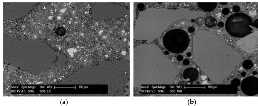
**Figure 2.** (a) Reference mixture containing no foaming agents or foams SEM images, (b) foamed concrete mixture SEM image. Reprinted/adapted with permission from Ref. [84]. 2015, Elsevier Science & Technology Journals.
