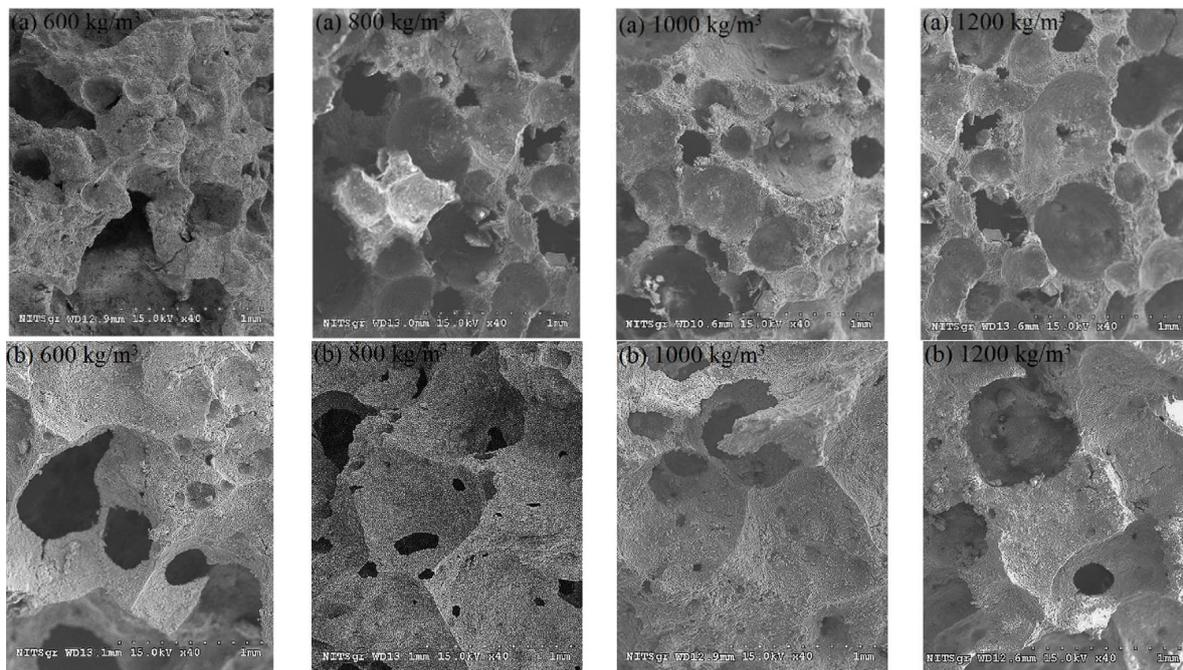
**Figure 10.** Microscopic images: (a) protein-based foam concrete, (b) synthetic-based foamed concrete. Reprinted/adapted with permission from Ref. [20]. 2021, Elsevier Science & Technology Journals.
