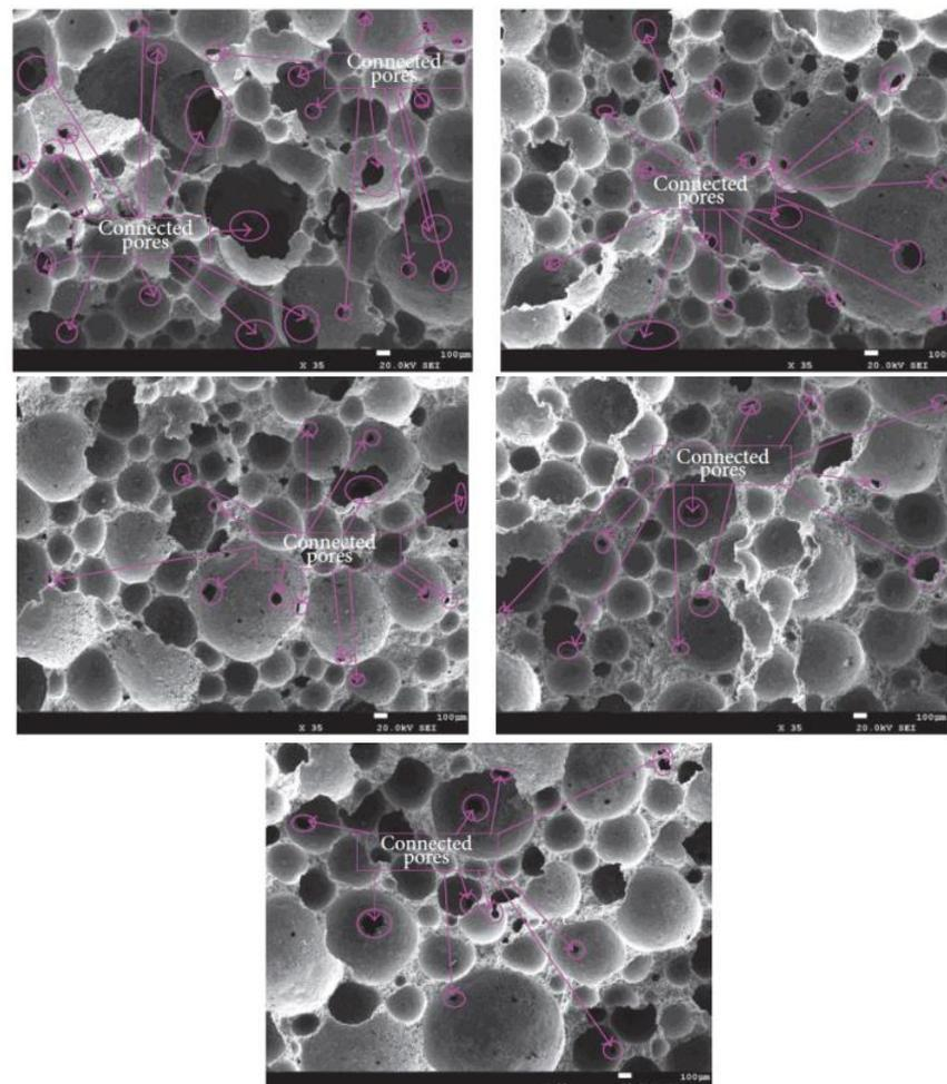
**Figure 4.** The effect of change in  $w/c$  ratio on pore structure [72].
