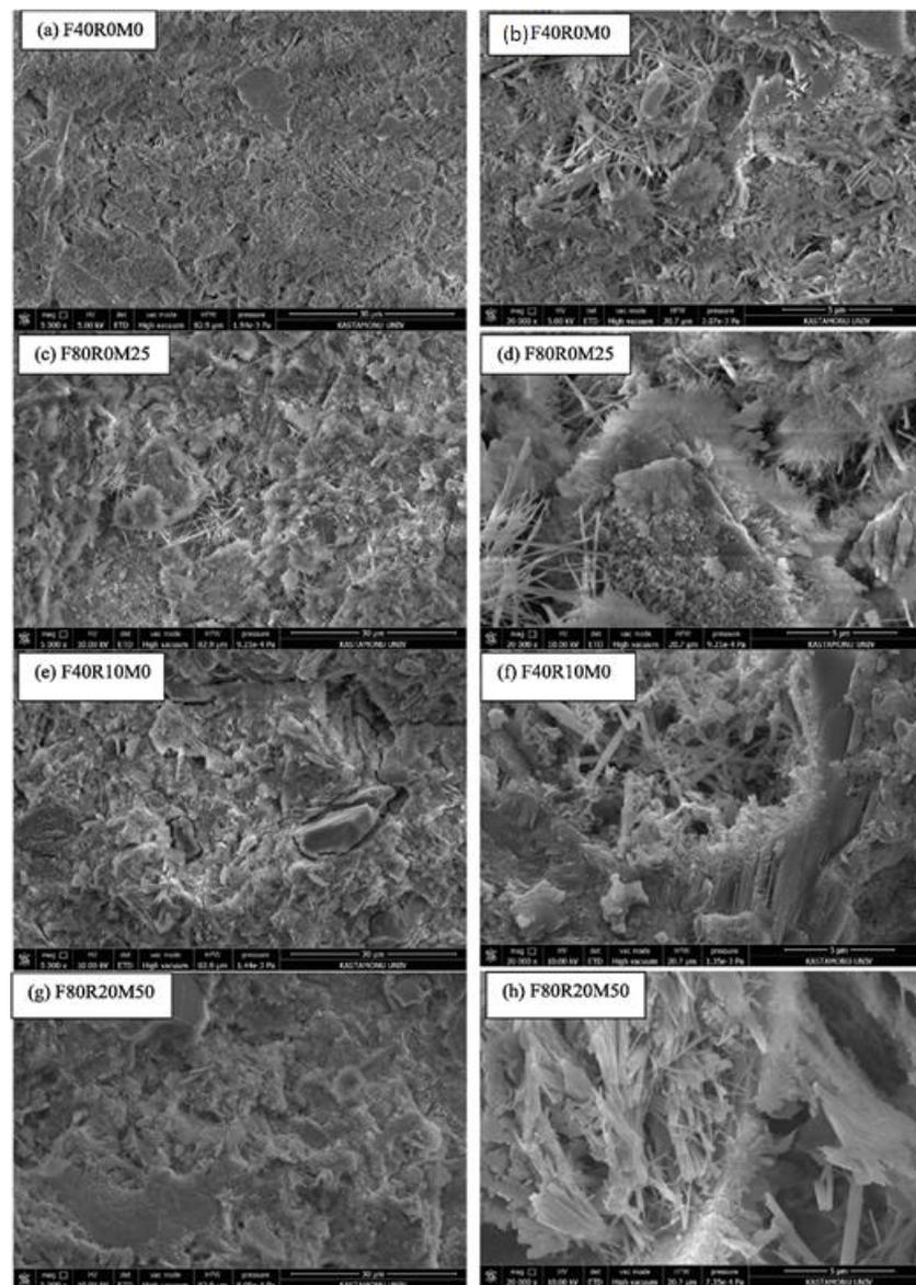
**Figure 5.** SEM images of foam concrete samples (F: foam content, R: rice husk ash, M: waste marble powder). Reprinted/adapted with permission from Ref. [18]. 2021, Elsevier Science & Technology Journals.
