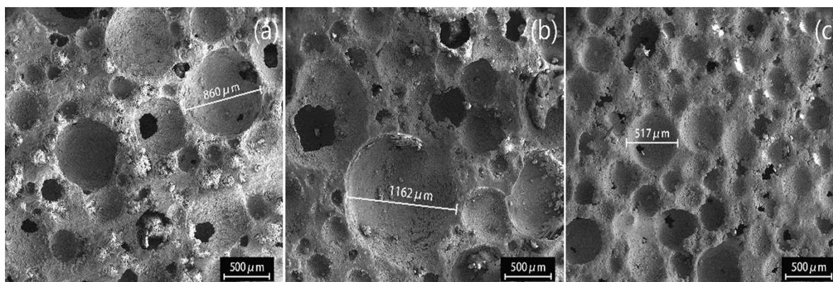
**Figure 9.** SEM images of foamed concrete at  $100\times$ : (a) AS, (b) PS, (c) SS. Reprinted/adapted with permission from Ref. [36]. 2018, Elsevier Science & Technology Journals.
