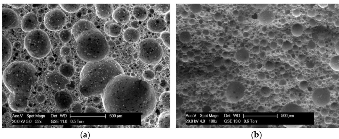
**Figure 8.** SEM images of foamed concrete ((a): concrete density =  $500 \text{ kg/m}^3$ , (b): concrete density =  $1000 \text{ kg/m}^3$ ). Reprinted/adapted with permission from Ref. [117]. 2013, Elsevier Science & Technology Journals.
