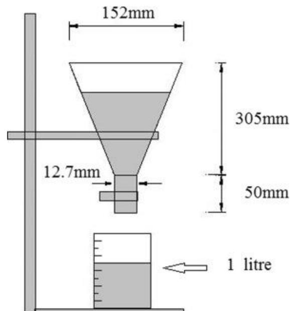
**Figure 1.** Modified Marsh cone [11].**Table 5.** Classifications of foam concrete with respect to the flow time [11].
