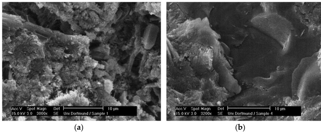
**Figure 3.** Microstructure of two foam concrete; (a)  $w/c = 0.60$ , containing no microsilica content; (b):  $w/c$  ratio = 0.35, with 10% microsilica content. Reprinted/adapted with permission from Ref. [116]. 2009, Elsevier Science & Technology Journals.
