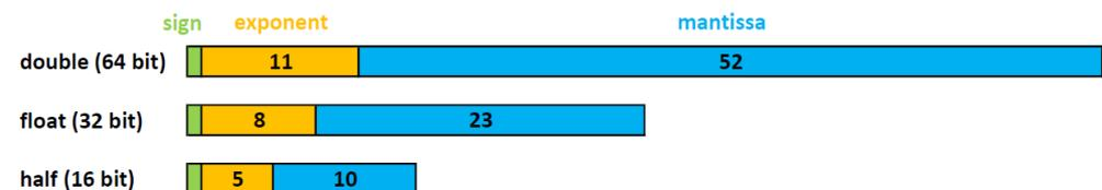
Figure 2. Encodings of the floating-point standard.
