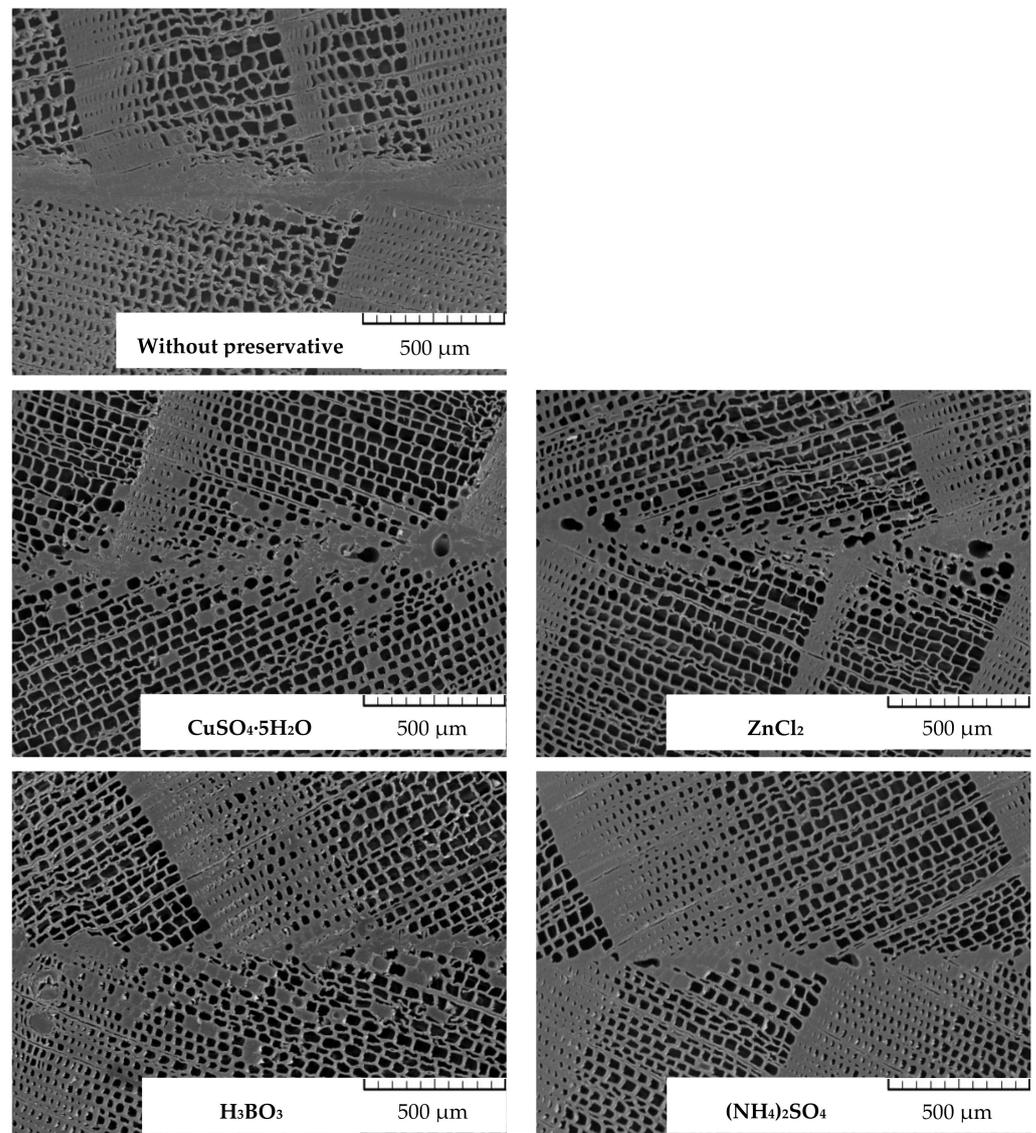
**Figure 5.** Microscopic analyzes of the “spruce wood—PUR glue” phase interfaces—without or with presence of inorganic preservative in the wood surface.
