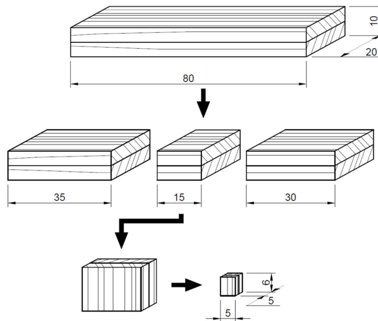
**Figure 2.** Preparation of the micro-plate (6 mm × 5 mm × 5 mm) for microscopic analysis of the “wood—PUR” interphase.
