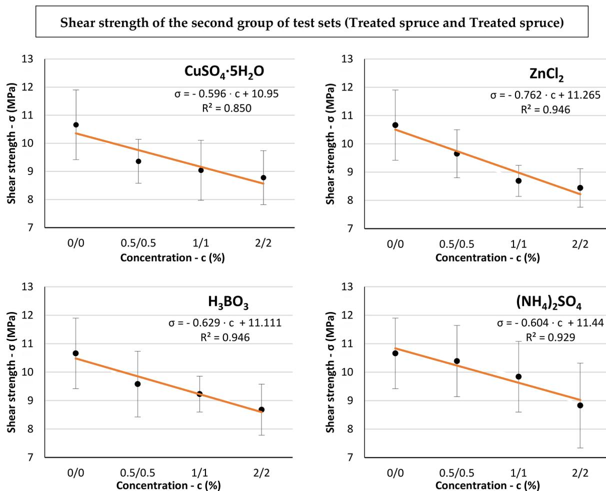
**Figure 4.** Linear dependencies between the shear strength of glued joints ( $\sigma$ ) and the concentration of a preservative ( $c$ ) in the second group of test sets “Treated spruce and Treated spruce”.
