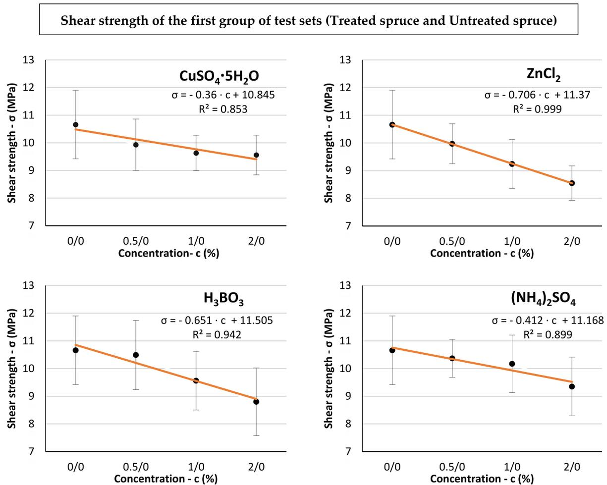
**Figure 3.** Linear dependencies between the shear strength of glued joints ( $\sigma$ ) and the concentration of a preservative ( $c$ ) in the first group of test sets “Treated spruce and Untreated spruce”.
