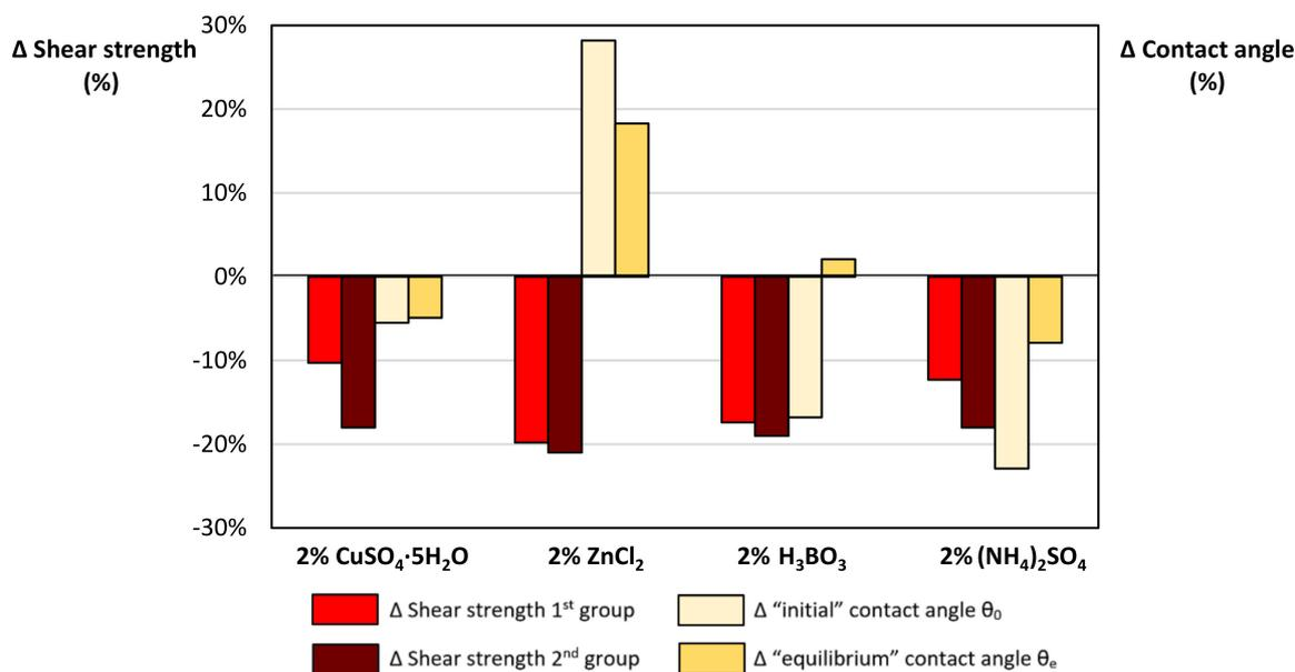
**Figure 6.** Comparison of the percentage change in the strength of glued joints ( $\Delta\sigma$ ) for the first and second group of test sets and the percentage changes in the contact angles ( $\Delta^\circ$ ) for the spruce wood specimens treated with the 2% solutions of inorganic preservatives.
