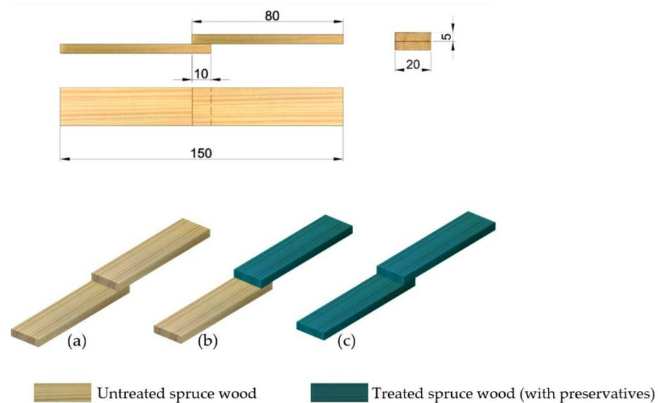
**Figure 1.** Dimensions of spruce wood specimens used for preparation of the control and test sets according to the standard EN 205 [49]. Dimensions are in mm. Composition of the sets is analogous with the sets prepared from themmally treated spruce woods [54]. Notes: (a) Control set, (b) First group of test set (Treated spruce and Untreated spruce), (c) Second group of test set (Treated spruce and Treated spruce).
