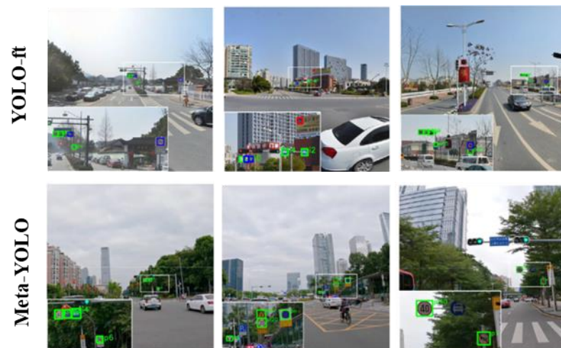
Figure 6. The visualization of novel class traffic signs by YOLO-ft and Meta-YOLO. Comparing with Meta-YOLO, YOLO-ft is inferior: b-boxes in the first columns are omitted; in the middle column they are wrong; in the last columns they are almost duplicated.
