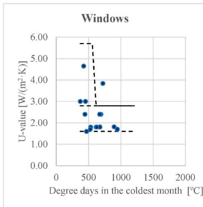
**Figure 3.** Law for the assignment of window U-values with heating degree days in the coldest month in each city.
