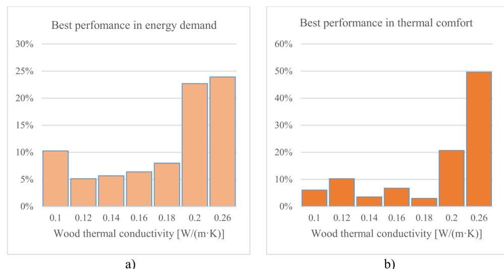
**Figure 9.** Percentage of cases in which each conductivity range was identified with (a) the lowest energy demand while meeting the minimum comfort requirement and (b) the greatest number of comfort hours.
