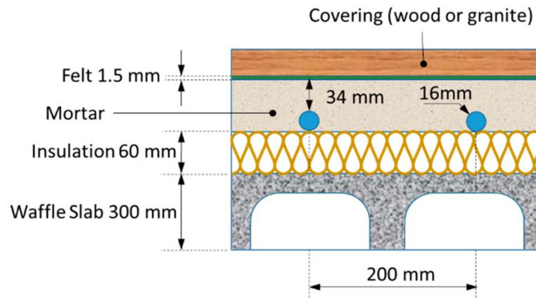
**Figure A2.** Radiant flooring layout.
