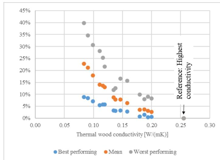
**Figure 10.** Effect of wood thermal conductivity on start-up lag time: percentage rise of start-up lag time relative to that of the floor with the highest wood covering conductivity.
