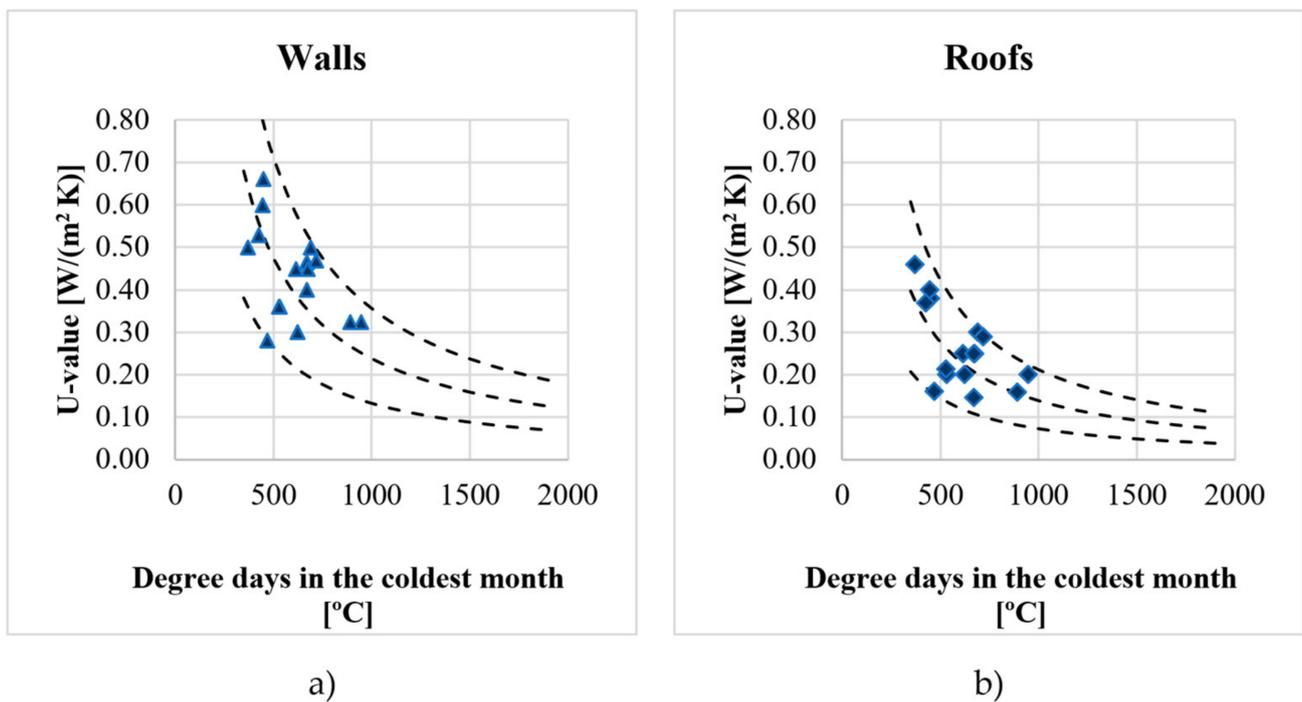
**Figure 2.** Law for the assignment of U-values with heating degree days in the coldest month in each city: (a) walls, (b) roof.
