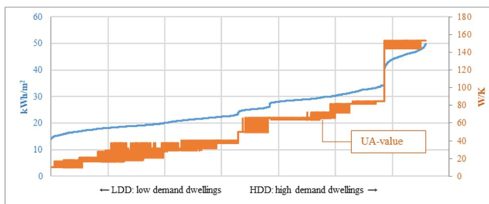
**Figure 8.** Energy demand and UA-value of outer enclosures for the dwellings of Moscow; in the part of the curve with a sharp increase in demand, around 35 kWh/m<sup>2</sup>, a sudden rise of the outer enclosure UA-value occurs due to the increase in the glazing percentage from 15% or 30% to 80%. This change would induce the steep rise observed.
