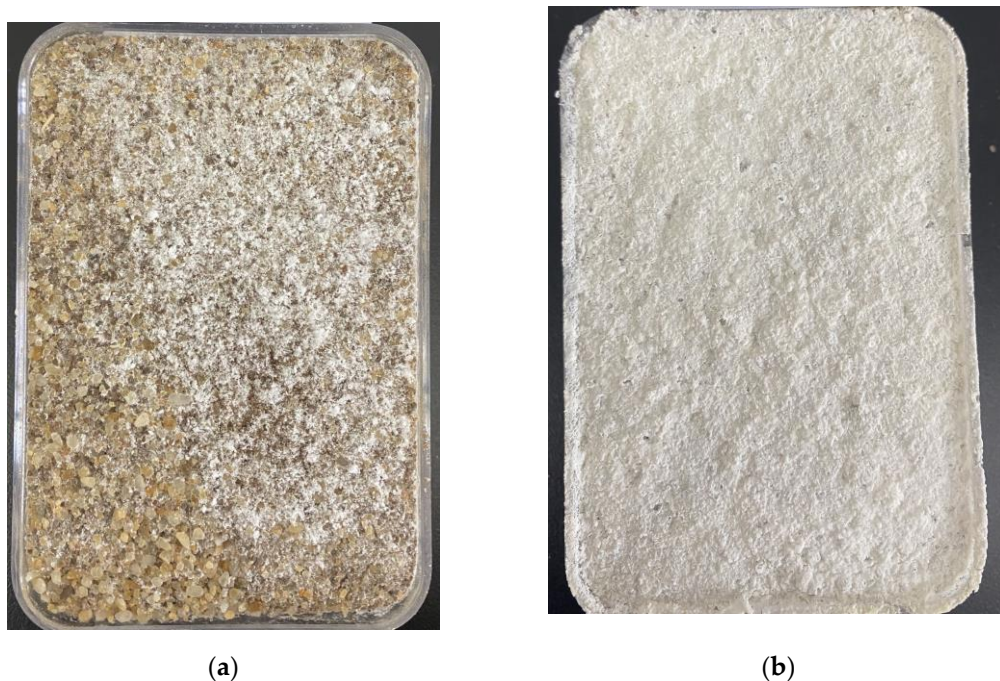
Figure 7. Specimen surface features: (a) with HPMC; (b) without HPMC.
