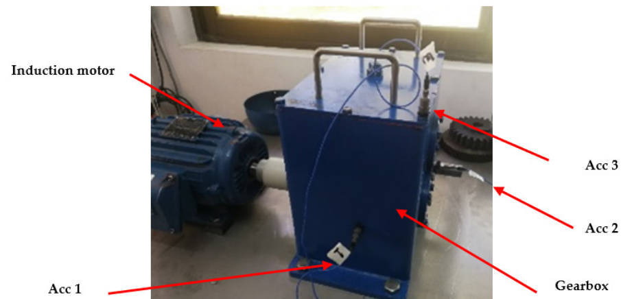
Figure 5. OMA's measurement set up for the gearbox with mounted accelerometers.
