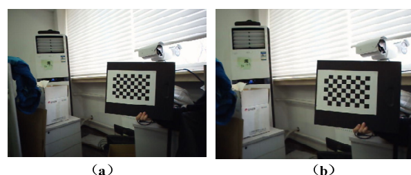
Figure 4. Checkerboard before and after distortion correction: (a) Before distortion correction; (b) After distortion correction.
