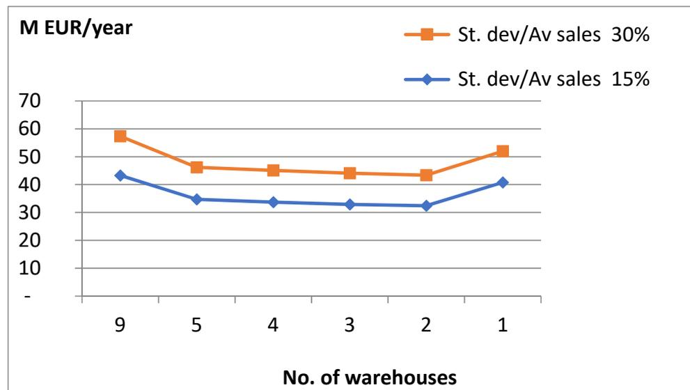
Figure 8. Impact of the number of warehouses and distances of deliveries on the total costs of distribution (Gaussian distribution, garments).
