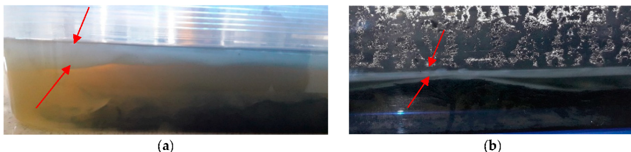
Figure 1. Thickness of bacterial cellulose (red arrows) cultured on: (a) SBR + CB; (b) SBR + cross-linking substances.
