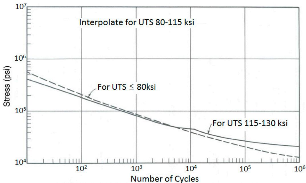
**Figure 13.** S–N curve for the material of the heater (ASTM A36, UTS = 58 ksi, or 400 MPa).
