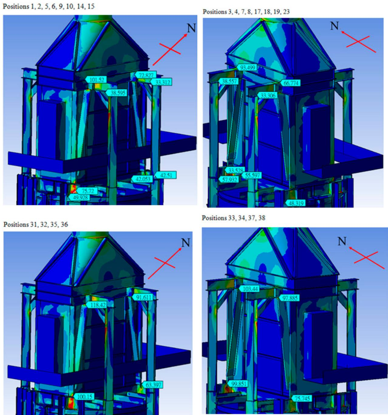
**Figure 7.** Results of finite element analysis for the present heater.
