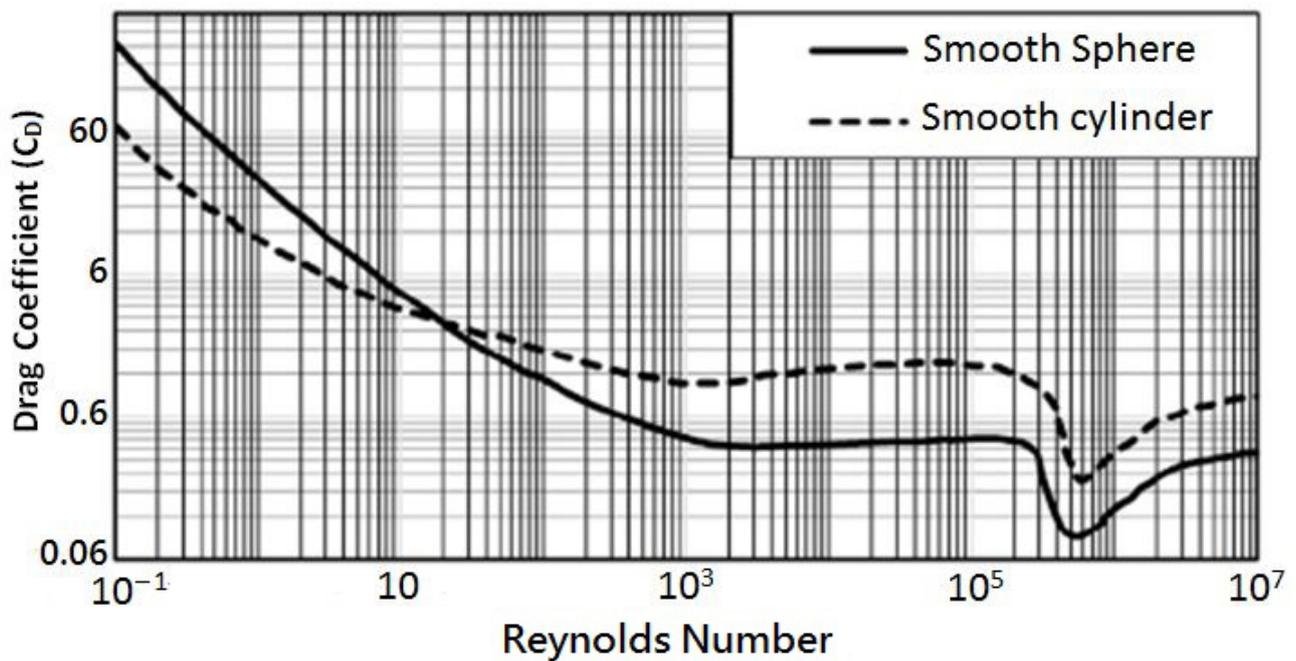
Figure 12. Drag coefficient of ideal sphere and circular cylinder by Schlichting.
