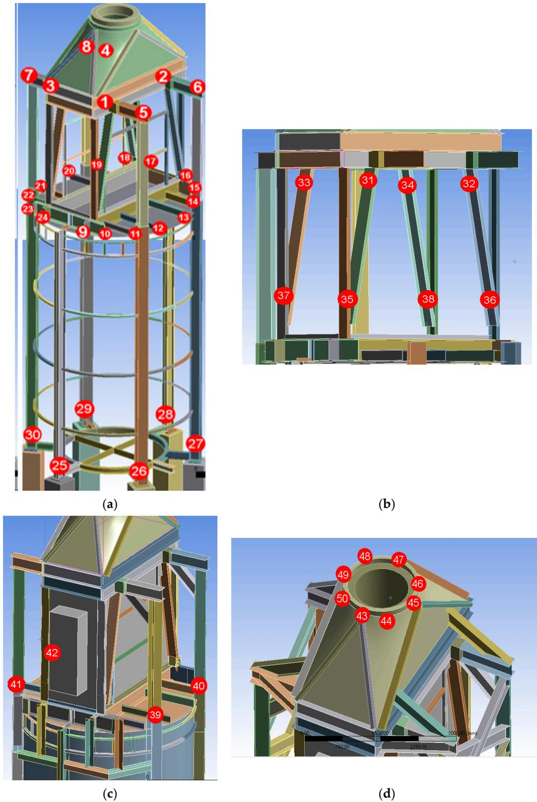
**Figure 4.** Illustration of the stress positions: (a) at the convection and radiation sections; (b) at the braces of the convection section; (c) at the junctions of the longitudinal beams; (d) near the root of the stack.
