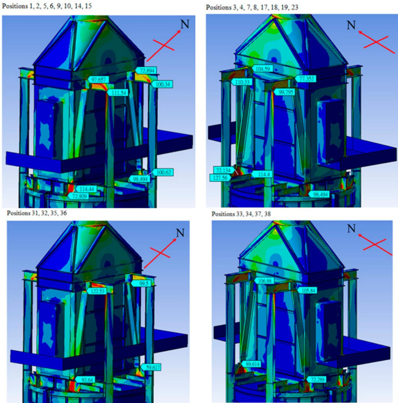
Figure 5. Results of finite element analysis for the heater before reinforcement.
