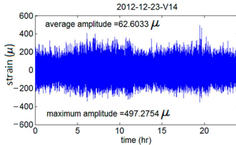
**Figure 3.** Measured strain at location V14 on the support frame.
