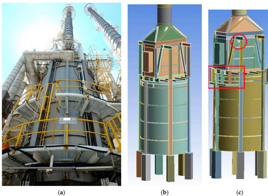
**Figure 2.** In Situ photograph and model of the heater. (a) in situ photograph, (b) model of original heater, (c) model of present heater (with reinforcement marked by circle and rectangle).
