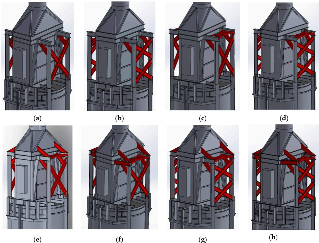
**Figure 8.** Eight different kinds of reinforcement methods for the support frame. (a) Case 1; (b) Case 2; (c) Case 3; (d) Case 4; (e) Case 5; (f) Case 6; (g) Case 7; (h) Case 8.
