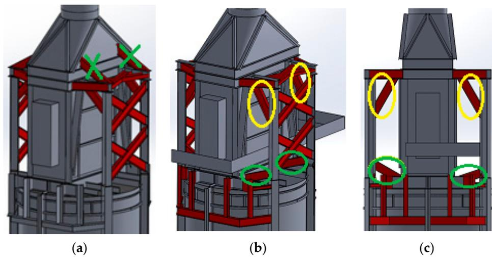
**Figure 10.** Numerical model for Case 9. (a) Case 8 (The braces with green marks are removed.); (b) Case 9 (The braces with green marks are added and the brace angles with yellow marks are changed, similar for (c)), (c) Case 9.
