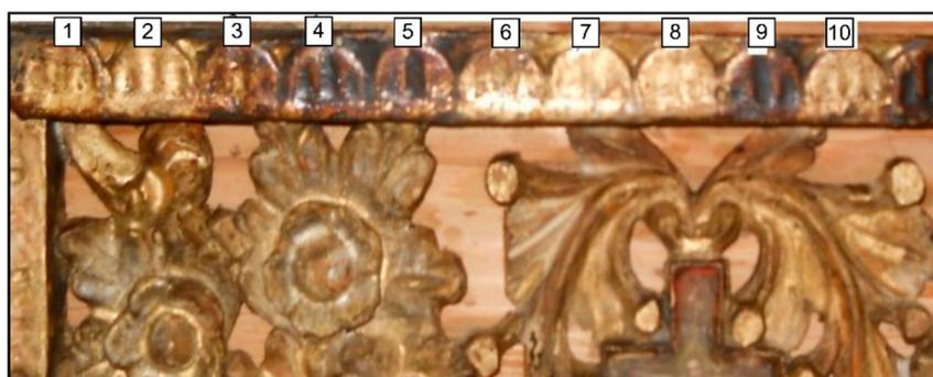
**Figure 12.** Washing tests for the gold gilded wood carving and embroidery with mono or mixed organic solvent solutions (E1–E10).
