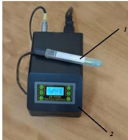
**Figure 5.** General view of a mobile device for creating cold plasma (CAP): 1—a replaceable module on the surface of which CAP is created; 2—hardware control block for DBD CAP creation modes.
