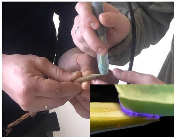
**Figure 6.** Processing (DBD CAP) a cut of a sweet cherry rootstock. The dielectric working surface of the replaceable module interacts with the cut surface and performs a sliding circular motion.
