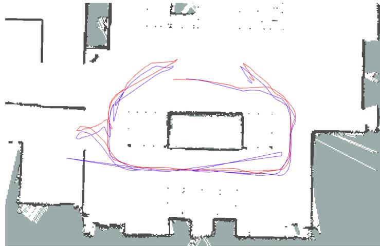
Figure 15. Path of robot, where the red lines indicate the path estimated by the robot and the blue lines indicate the paths measured by the MoCap system.
