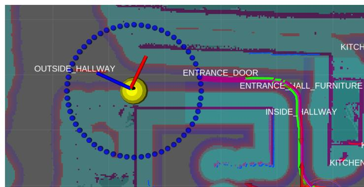
**Figure 3.** Person following example. The yellow sphere represents the person position, blue spheres represent the possible positions the robot could be at the desired distance to the person and the purple line is the path the robot chose from its position to the chosen target position.
