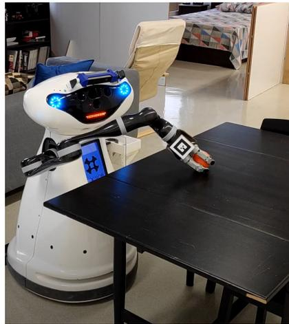
**Figure 1.** The Mbot mobile robot at the ISR/IST ERL certified test bed performing a pick and place operation.
