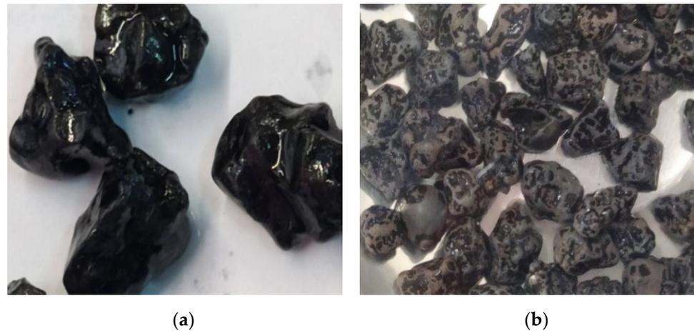
**Figure 4.** Examples of SSA aggregates surface covered with bitumen: (a) at the beginning of the affinity test; (b) after 24 h of exposure to test conditions.
