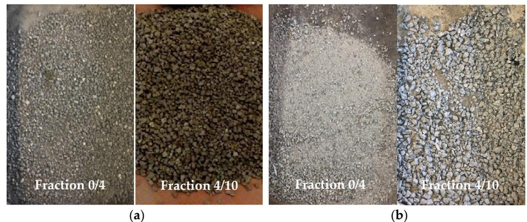
**Figure 1.** Materials used in this work: (a) steel slag aggregates (SSA) and (b) natural aggregates (NA).
