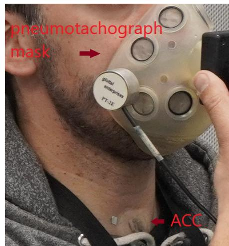
**Figure 6.** Experimental setup with oral airflow (pneumotachograph) mask and accelerometer sensor (ACC) on neck-surface location.
