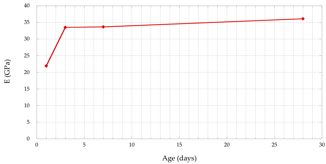
Figure 11. Evolution of the modulus of elasticity of FRC with age.
