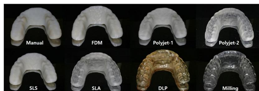
**Figure 1.** Occlusal splint fabricated with manual method, various 3D printing technologies, and the milling method.
