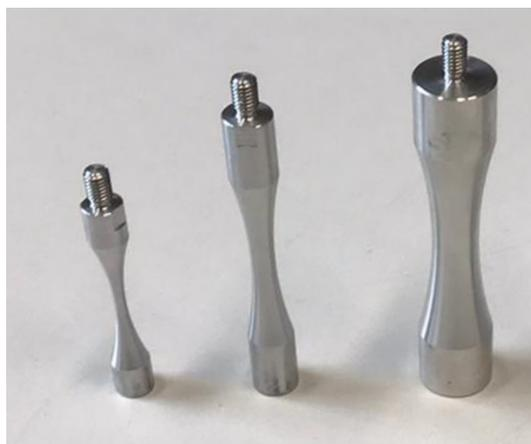
**Figure 2.** The three different investigated hourglass-specimens.
