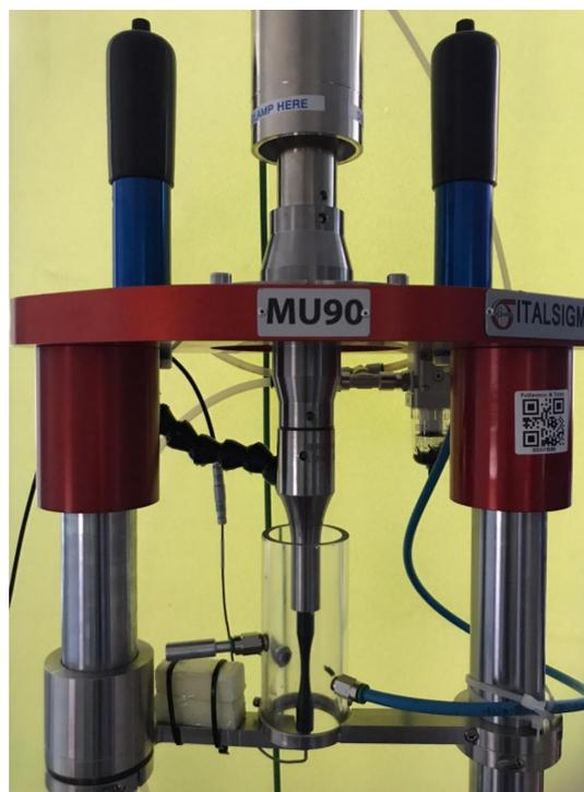
Figure 1. Ultrasonic fatigue testing machine MU90.
