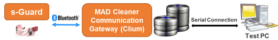
Figure 7. Experiment model of s-Guard Bluetooth communication performance.
