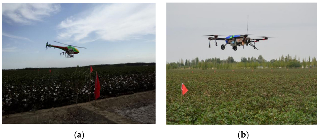
Figure 5. HY-B-15L single-rotor plant protection unmanned helicopter for cotton defoliant spray (a) and TXA616 plant protection UAV for rice growth regulator spray (b) [46].
