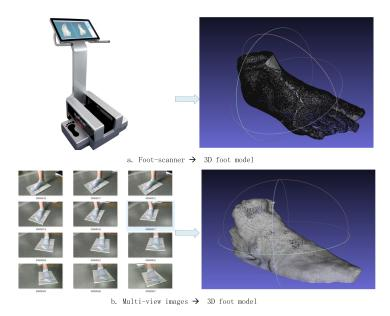
Figure 8. 3D foot model comparison of foot-scanner and Multi-images.
