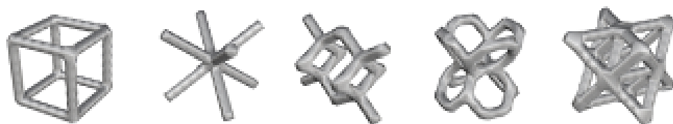
Figure 1. Strut-based unit cells. From left to right: grid, X (or BCC), diamond, vintiles, octet. Made using IntraLattice [82].
