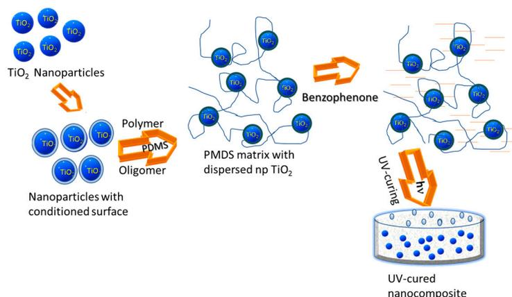
**Figure 2.** Preparation of the PDMS- $\text{TiO}_2$  nanocomposites applying a blending route. PDMS—polydimethylsiloxane.
