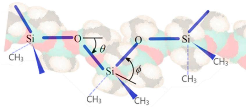
**Figure 1.** Polydimethylsiloxane (PDMS) backbone.
