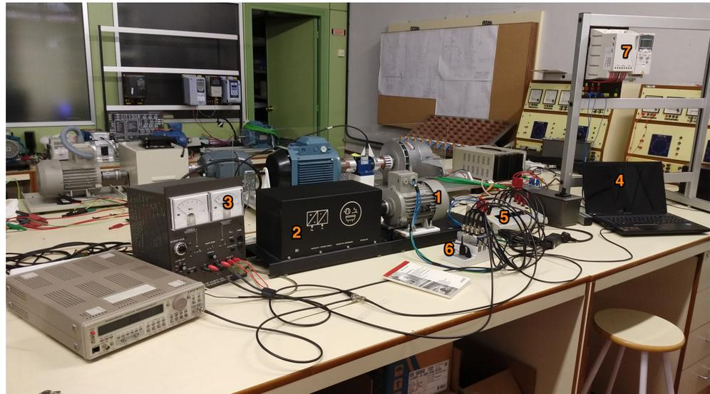
**Figure 3.** Elements of the test bench: (1) Induction motor; (2) Magnetic powder brake; (3) Brake control unit; (4) Laptop; (5) Custom-made board of sensors; (6) CompaqDAQ by National Instruments; (7) ABB inverter.
