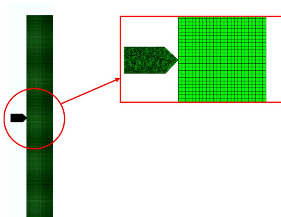
Figure 4. Meshing of 7.62 AP steel bullet core and target plate.
