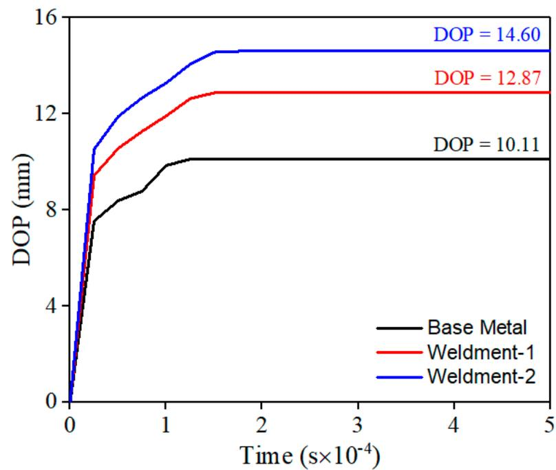
Figure 10. Depth of Penetration vs. Step time.
