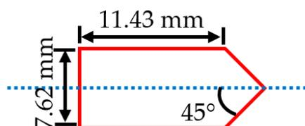
**Figure 2.** Schematic diagram of 7.62 AP Bullet steel core [13].
