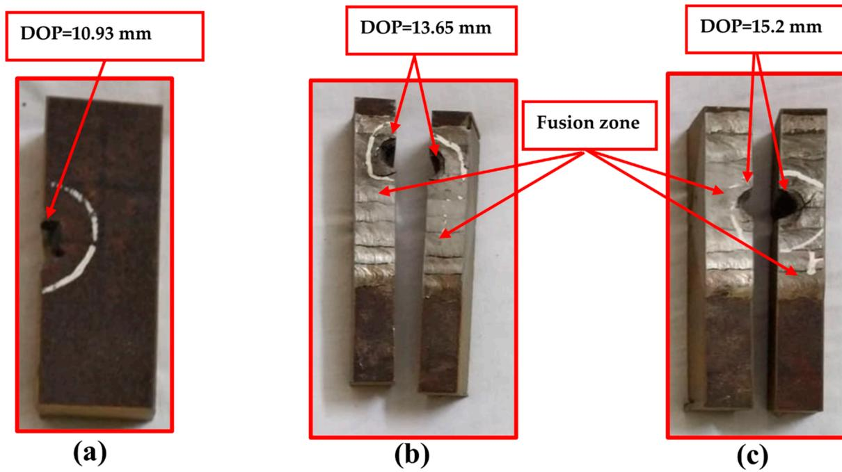
Figure 7. 7.62 AP bullet penetration cut section of (a) base metal, (b) weldment-1, (c) weldment-2.
