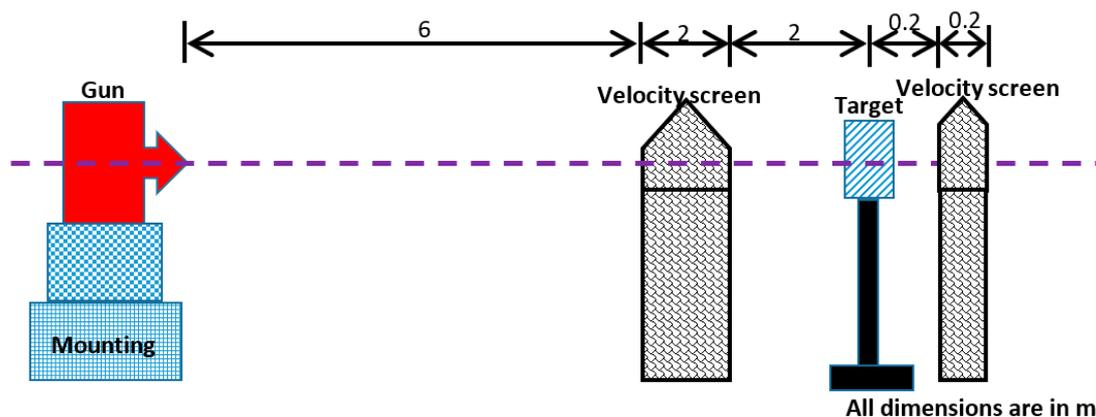
**Figure 1.** Schematic diagram of bullet penetration test.
