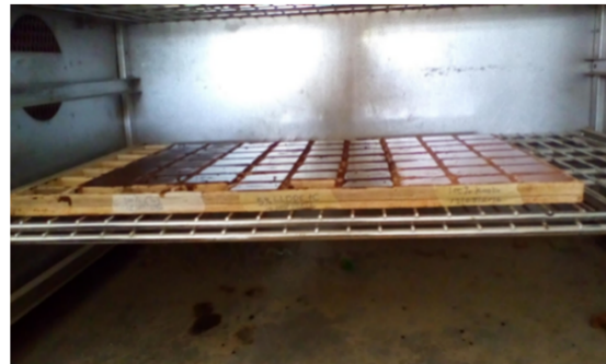
Figure 2. Geopolymer ceramics cured in oven.
