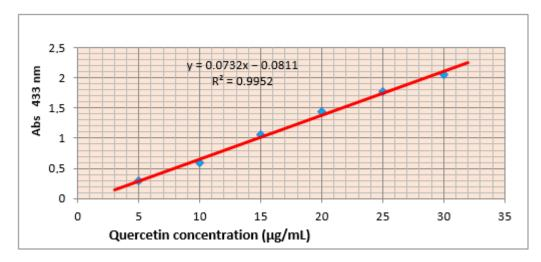
Figure 2. Quercetin calibration curve used for total quantification.
