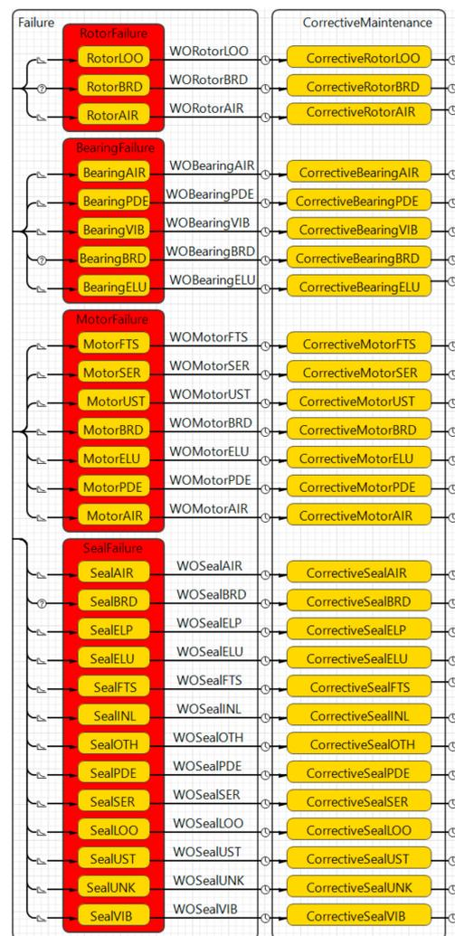
Figure 4. Failure events and corrective maintenance.
