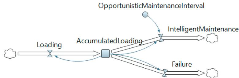
Figure 5. Loading model using systems dynamics.
