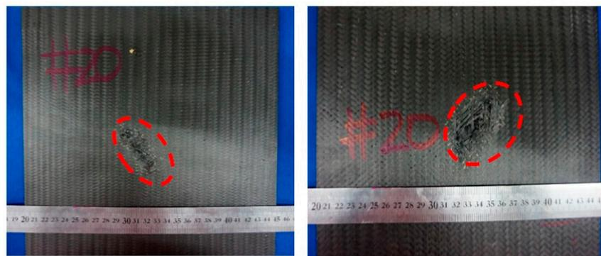
(b) CFRP-3 test,  $V_i = 157\text{ m/s}$ , room temperature.
