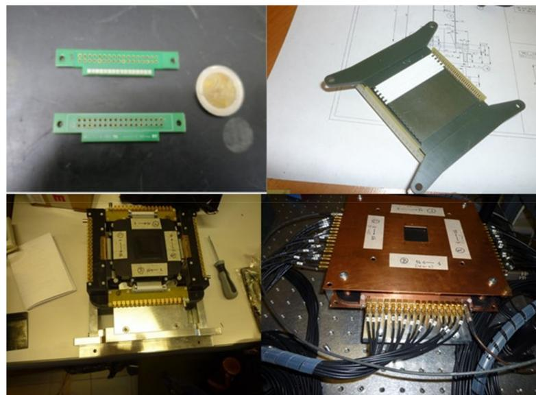
**Figure 6.** Top left panel: Picture of the PCBs with 1 mm SiPM soldered on. Top right panel: Picture of one fiber holder with some 1 mm fibers inside. The two PCBs with SiPM are shown. Bottom left panel: Mechanics layout of the 1 mm beam hodoscope. Bottom right panel: Image of the mounted detector. Signal/power cables are fanned out through the feedthrough along the lateral side of the structure.
