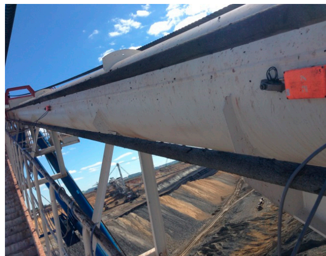
Figure 11. Location of AE sensors on a dragline boom.
