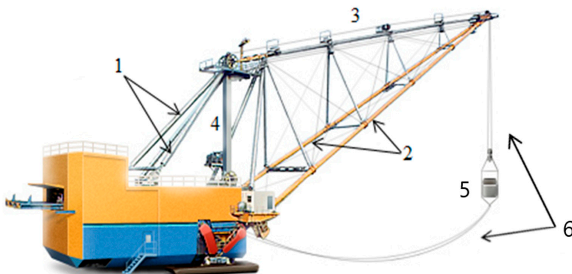
Figure 1. Basic components of a dragline ESH-20.90: 1—back legs, 2—boom, 3—hoist rope, 4—mast, 5—bucket, 6—dragrope.
