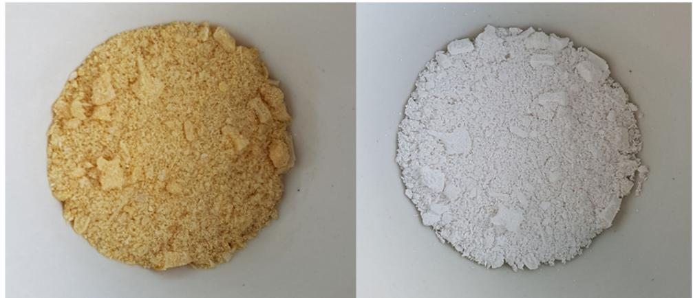
**Figure 2.** Crushed fish bones before and after thermal treatment.
